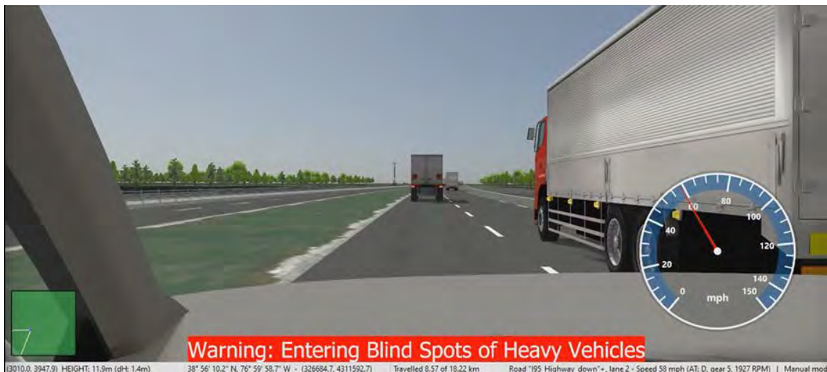
Figure 11: BSW triggered in the Area #3 at the Left Side of the Truck
