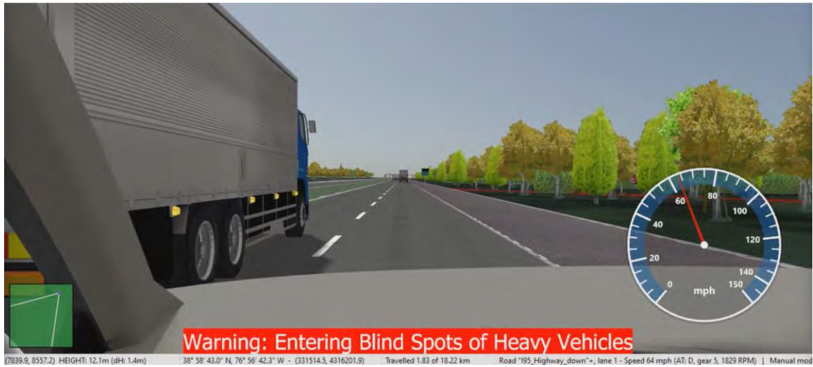
Figure 10: BSW-H triggered in the Area #2 at the Right Side of the Truck
