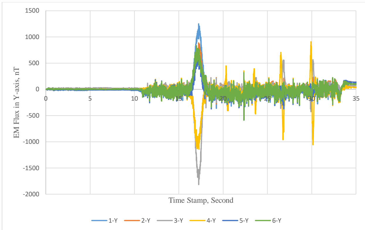
Figure 55. Graph. Referenced EM Flux Signal after initializing initial reading value at zero and gradiometer processing for sensors Y-axis (Case #1).
