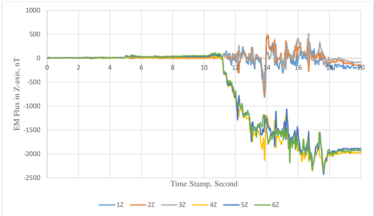
Figure 119. Graph. High-frequency filtered EM flux for sensors in Z-axis (Case #1).
