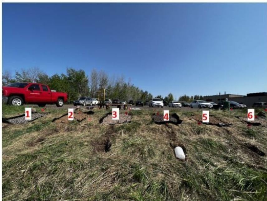
Figure 6.2. The six new plots were constructed on May 25, 2023. The media used were as follows: 20% peat/biochar with 80% recycled concrete aggregate (plots 1 & 4), 20% degritter with 80% dredge sediment (plots 2 & 5), and 20% sawdust with 80% recycled concrete aggregate (plots 3 & 6). These new plots are positioned adjacent to the previously established seven experimental plots (next to plot 6).
