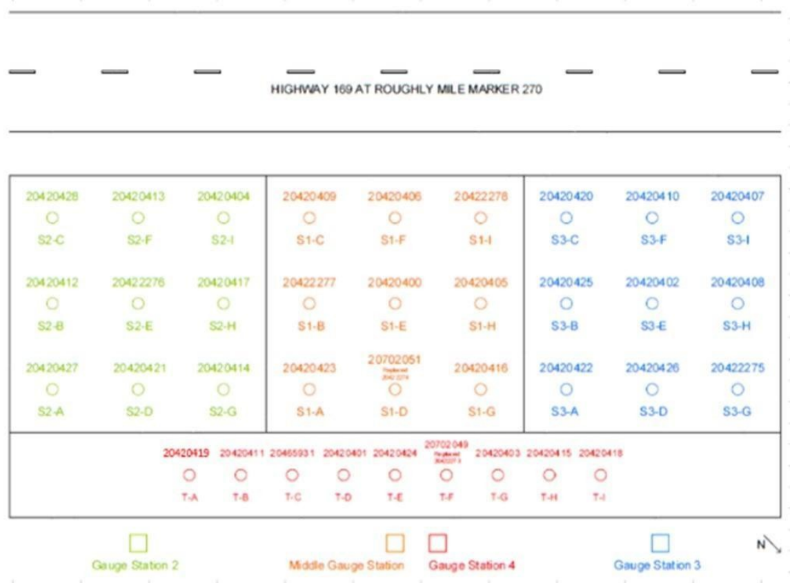
Figure 6.4. The layout of the sensors at Eagle's Nest site in 2022/23 (adapted from Cai et. al, 2021).
