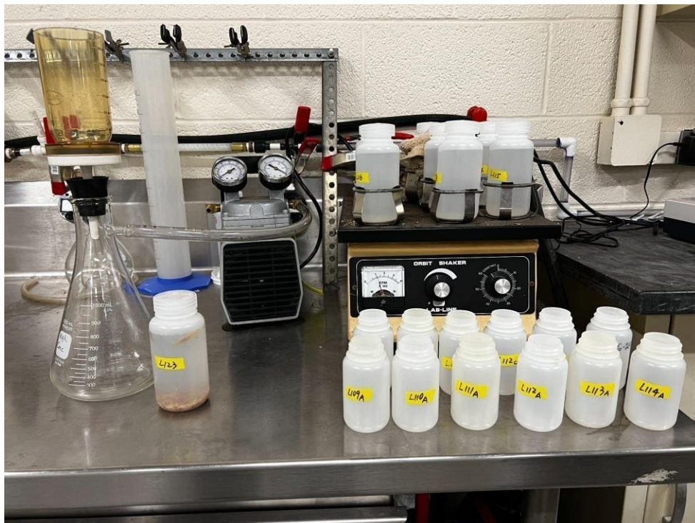
Figure 3.13. The picture of the batch testing apparatus, including the shaking table, vacuum pump, and filtration funnel.
