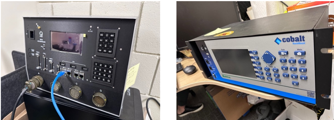
Figure 2: Traffic Signal Controllers. Q-Free XN-2 Controller (left) and Econolite Cobalt Controller (right) in the signal testbed at the University of Minnesota.
