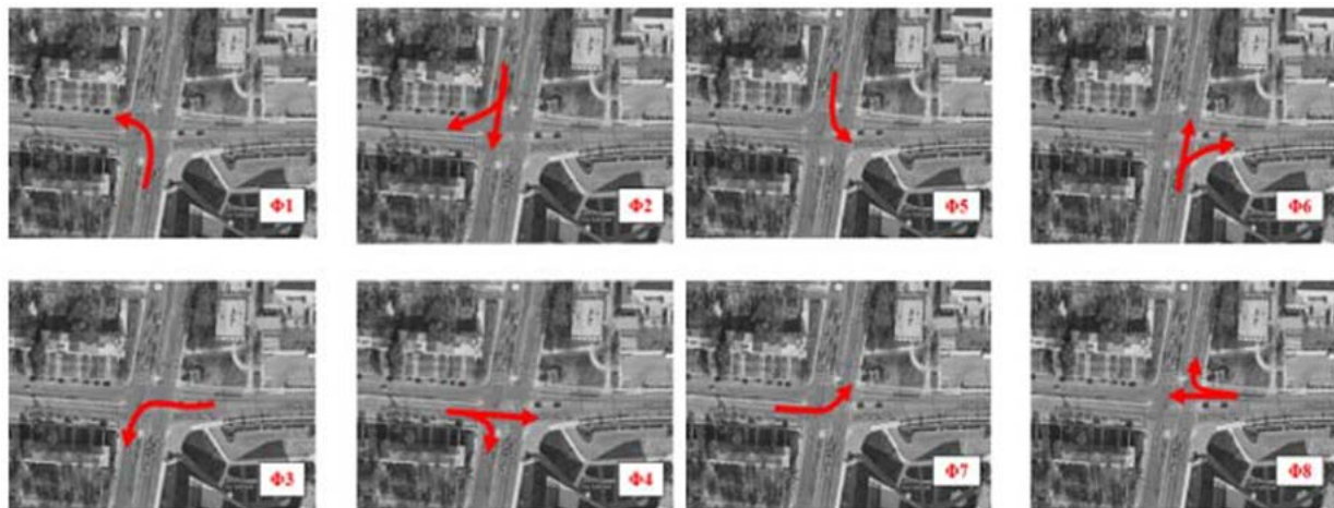
Figure 18 Different Phases of The Traffic Signal
