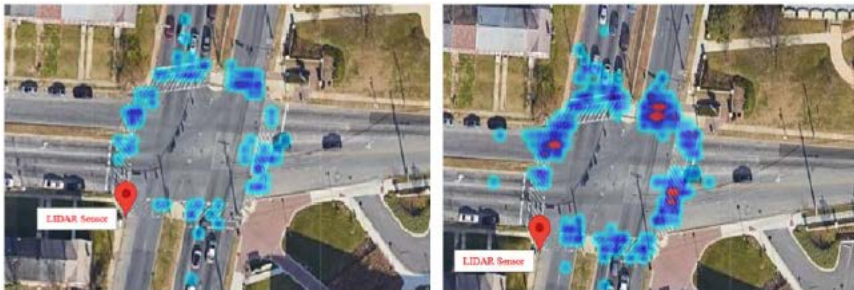
Figure 20 Vehicle-Pedestrian Conflicts Heat Map in July (left figure) and August (right figure)
