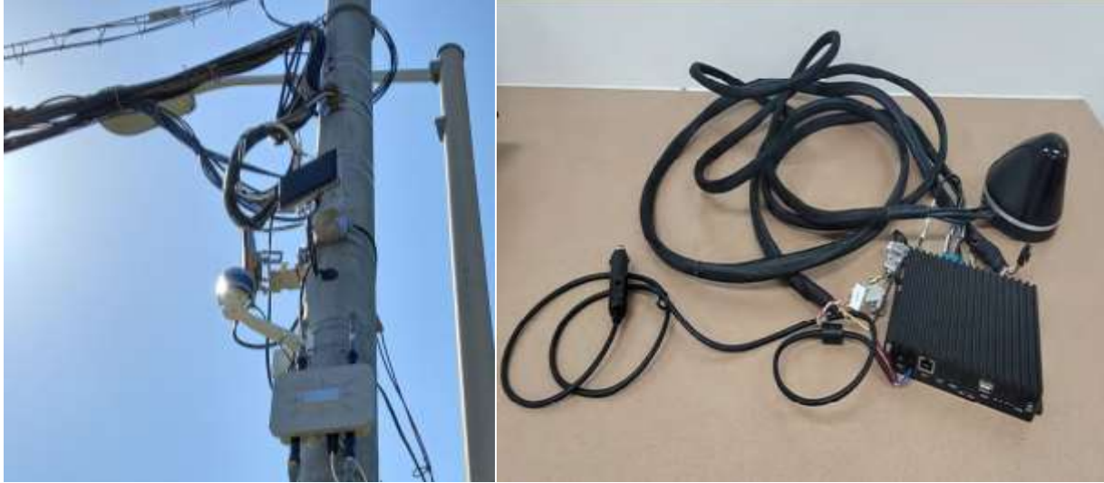
Figure 2 LiDAR Sensor, RSU, and OBU Setup on the Morgan State University CAV Testbed
