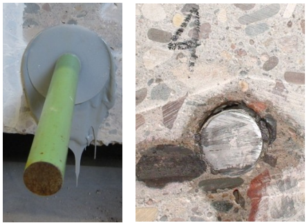
Adhesive Sample Test Hole #4 - Single Dip Two Part Epoxy / Hand Mixed
