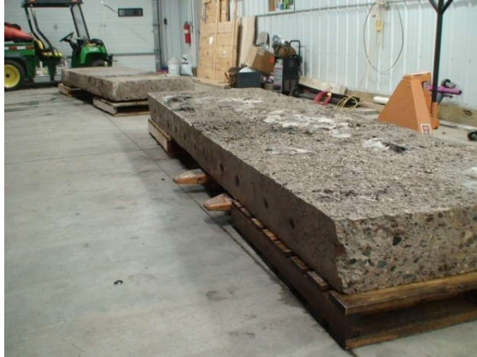
Figure 3. Concrete Panels after gang drilling Process
