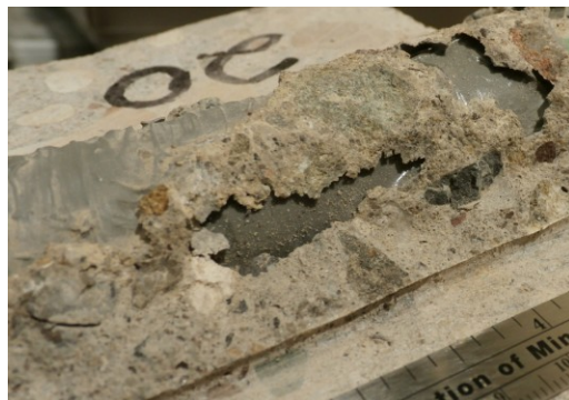
Adhesive Sample Test Hole #20 - Epoxy filled hole and applied bead of epoxy to dowel
