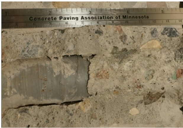
Adhesive Sample Test Hole #11 - Epoxy filled hole and applied bead of epoxy to dowel
