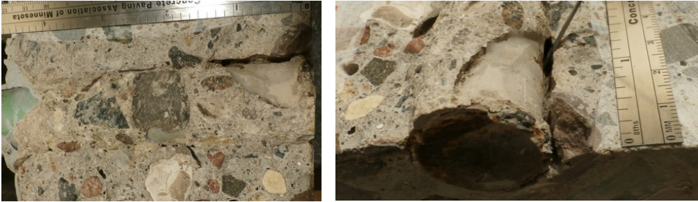
Adhesive Sample Test Hole #1 - Epoxy Dowel Bar Rotating Together Mixing Process
