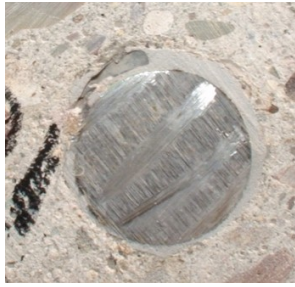
Adhesive Sample Test Hole #21 - Poly-Grip is a two-component epoxy – 25 ‘Pumps’ of adhesive
