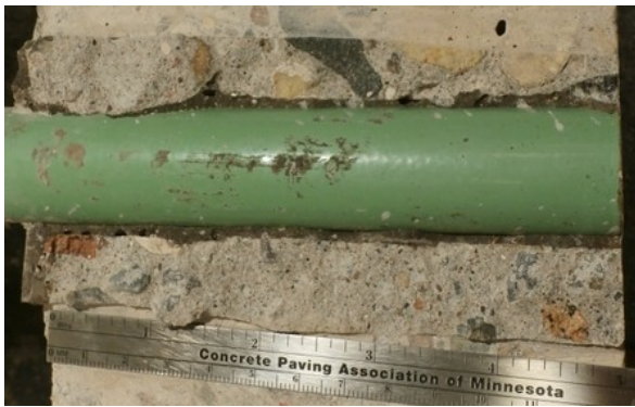
Adhesive Sample Test Hole #29 - Cementitious Anchoring Capsule Grout
