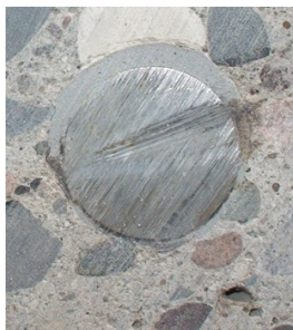
Adhesive Sample Test Hole #22 - Poly-Grip is a two-component epoxy – 20 ‘Pumps’ of adhesive
