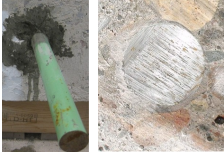
Adhesive Sample Test Hole #28 - Cementitious Anchoring Capsule Grout
