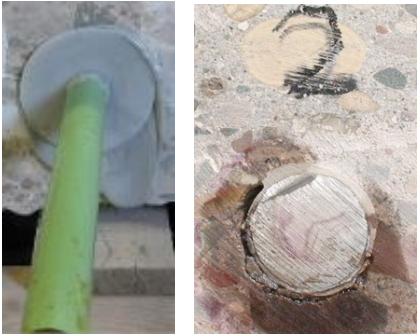
Adhesive Sample Test Hole #2 - Epoxy Dowel Bar Rotating Together Mixing Process
