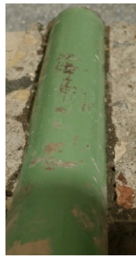
Adhesive Sample Test Hole #29 - Cementitious Anchoring Capsule Grout
