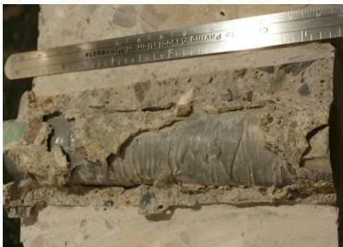
Adhesive Sample Test Hole #20 - Epoxy filled hole and applied bead of epoxy to dowel
