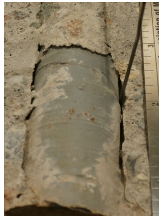
Adhesive Sample Test Hole #11 - Epoxy filled hole and applied bead of epoxy to dowel
