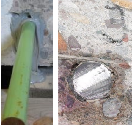
Adhesive Sample Test Hole #3 - Single Dip Two Part Epoxy / Hand Mixed
