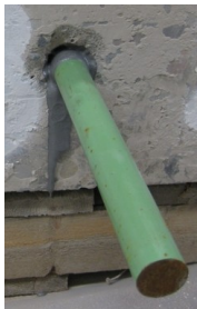
Adhesive Sample Test Hole #23 - Poly-Grip is a two-component epoxy – 20 ‘Pumps’ of adhesive
