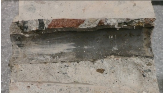
Adhesive Sample Test Hole #26 - Cementitious Anchoring Capsule Grout
