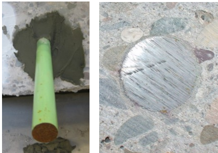
Adhesive Sample Test Hole #7 – Non-Shrink Grout, used past recommended application time
