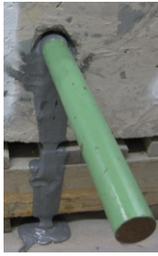
Adhesive Sample Test Hole #21 - Poly-Grip is a two-component epoxy – 25 ‘Pumps’ of adhesive
