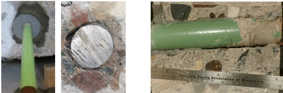
Adhesive Sample Test Hole #7 – Non-Shrink Grout, used past recommended application time
