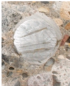
Adhesive Sample Test Hole #23 - Poly-Grip is a two-component epoxy – 20 ‘Pumps’ of adhesive
