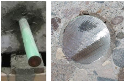
Adhesive Sample Test Hole #33 – Non-Shrink Grout
