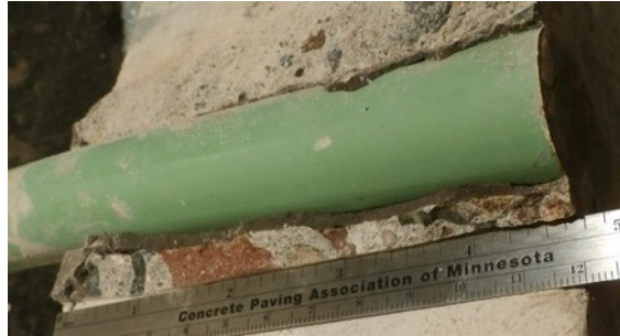
Adhesive Sample Test Hole #26 - Cementitious Anchoring Capsule Grout
