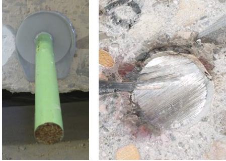
Adhesive Sample Test Hole #6 - Double Dip Two Part Epoxy / Hand Mixed
