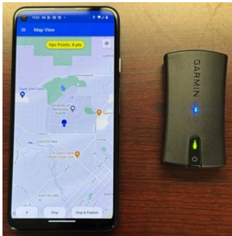
Figure 4.7 External GPS receiver device along with the Android phone.
