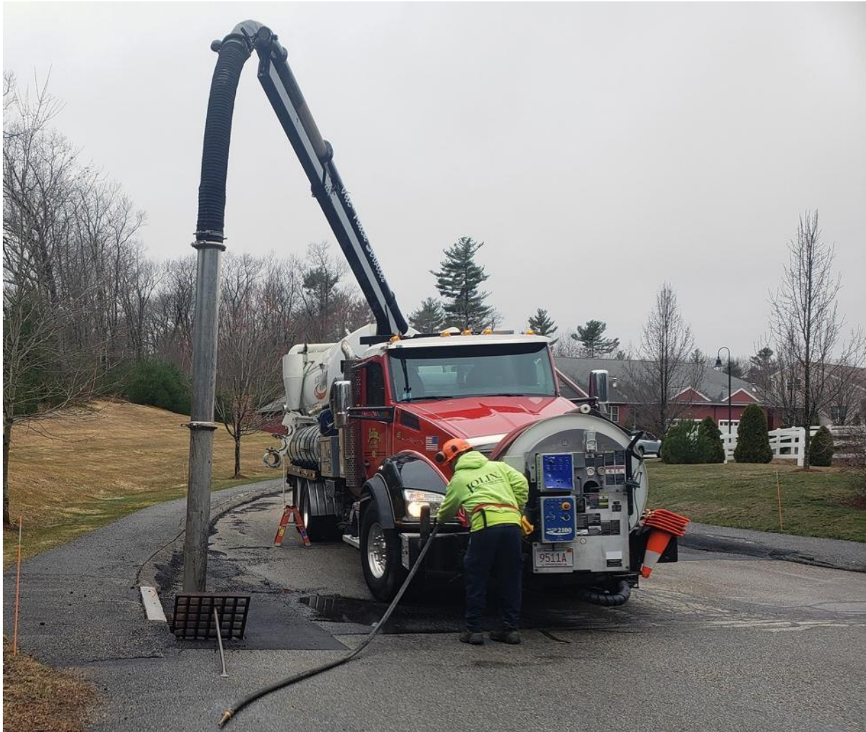
Figure 3-1: Example of a vector truck in operation. Photo: www.jolinpavingandexcavating.com
