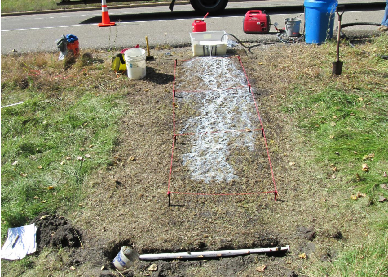
Figure 6-5: Field tests on the performance of a filter strip. Photo: John Gulliver.
