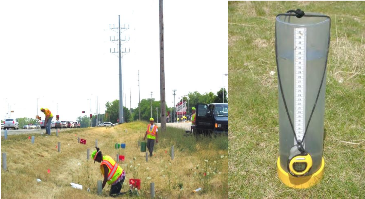
Figure 1-2: Multiple infiltration capacity tests at a roadside swale (left) using the MPD Infiltrometer (right). Photos: John Gulliver.
