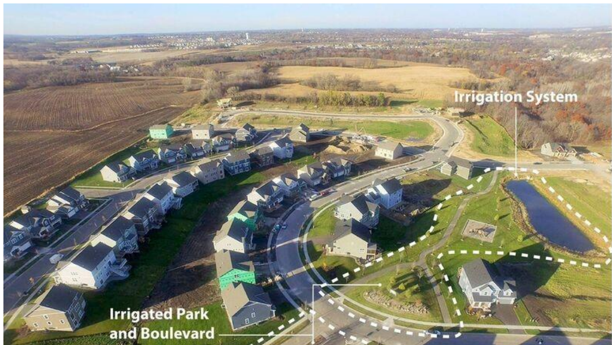
Figure 8-6: Carver County stormwater harvesting site. Photo: DR Horton Homes.
