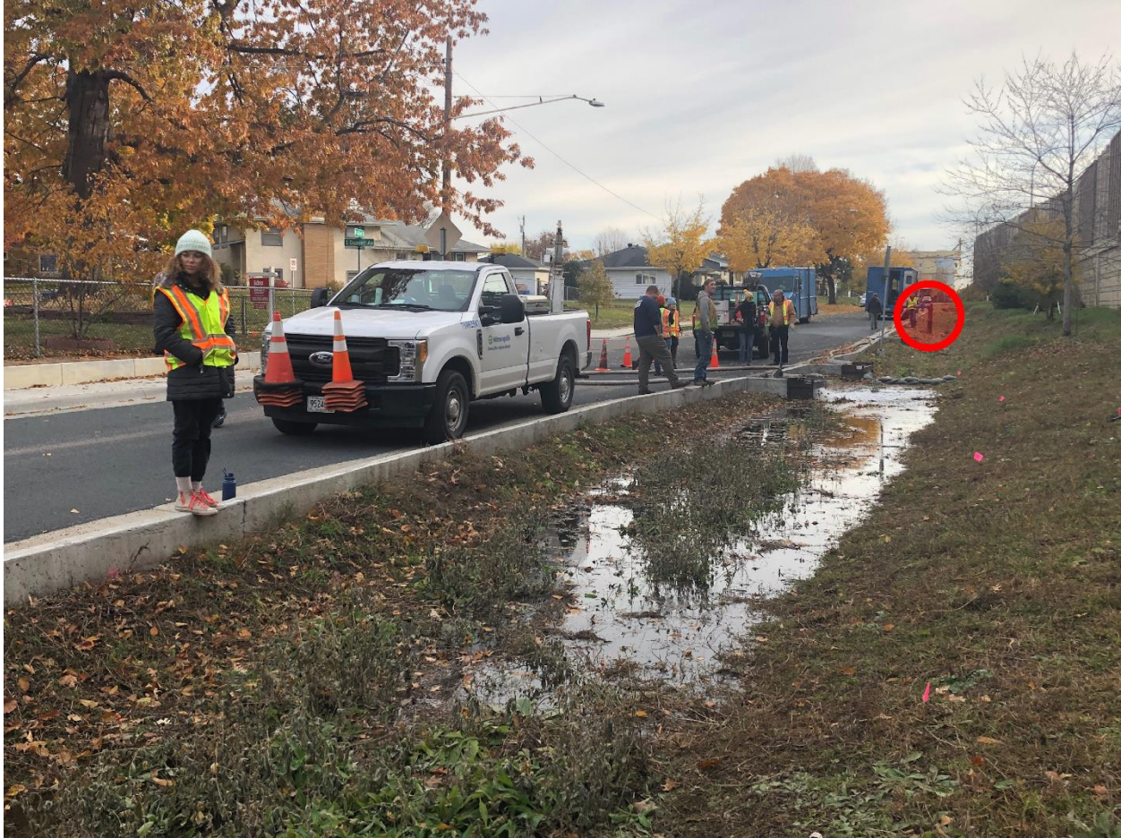
Figure 1-3: Synthetic runoff test using a metered fire hydrant (red circle) at a bioretention practice. After water fills the bioretention practice, the recession of the water surface is measured over time. Photo: John Gulliver.
