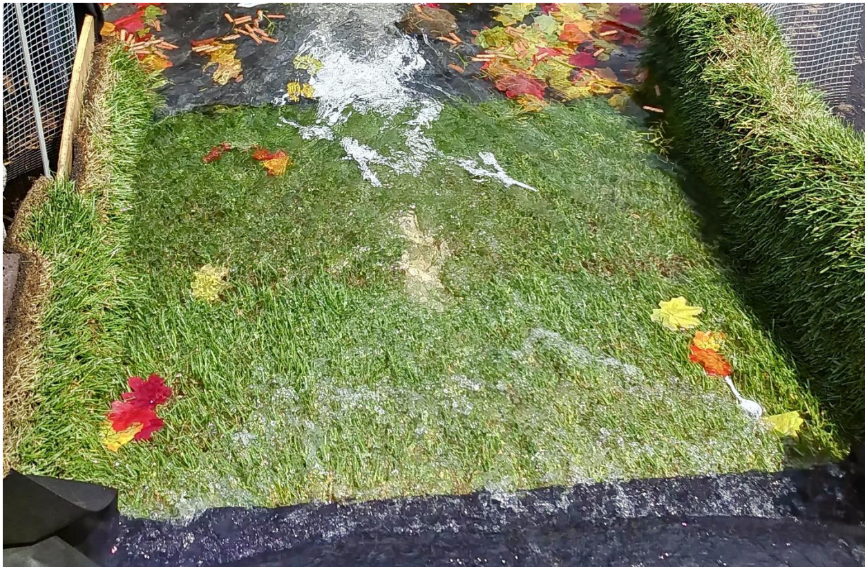
Figure 6-2: Sheet flow over rain garden pretreatment section. Photo: Andy Erickson.
