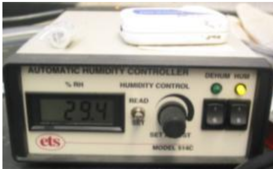
Figure A7. The ETS control box associated with the humidity conditions in the Coy Chamber.
