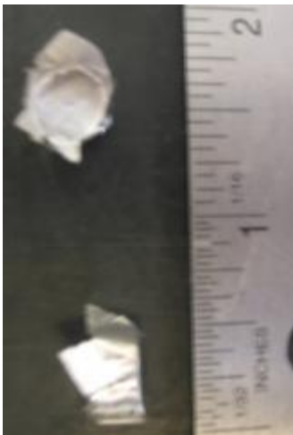
Figure A9. Aluminum foil cup top view (top) and side view (bottom) with ruler for scale.
