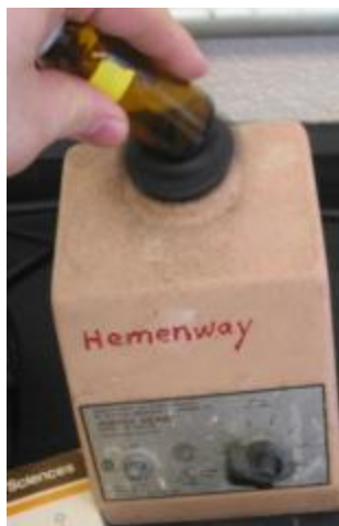
Figure A2. How to hold impinger sample on vortexer.
