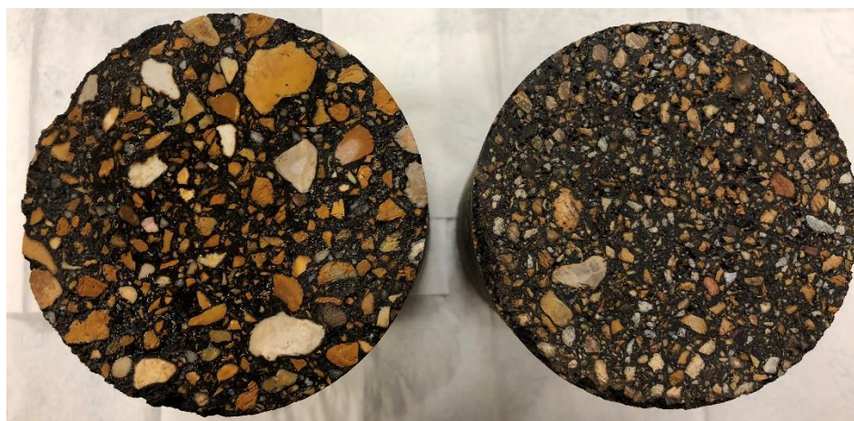
Figure 1. 12.5-mm NMAS mixture (left) next to 4.75-mm NMAS mixture (right)
