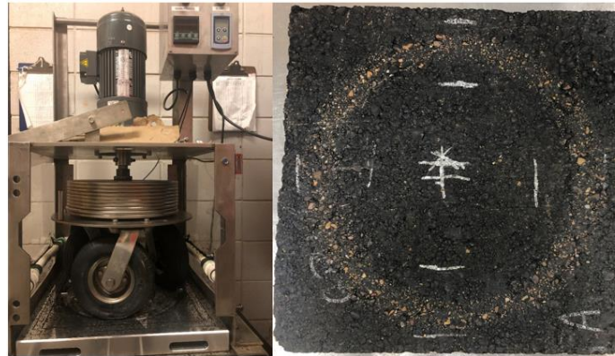
Figure 6. Three wheel polisher and polished slab
