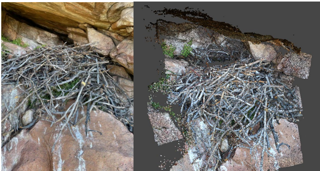
Figure 2.18 SfM (left) and Lidar (right) based models of a raptor nest in Staunton State Park in Colorado.
