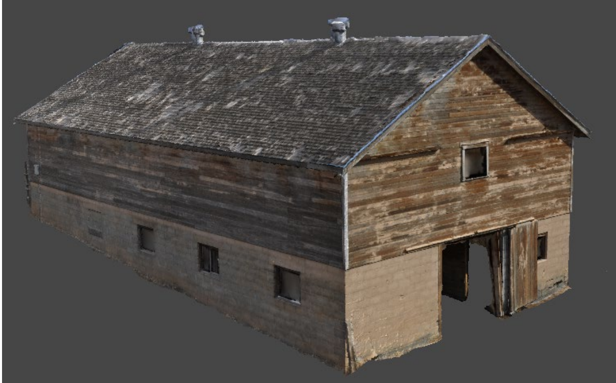
Figure 2.12 A still shot of the rendered image from SfM software with excellent resolution for a relatively small number of still images.
