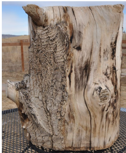
Figure 2.1 An image of a tree stump used for imaging and inspection models. This structure was selected because of the wide variety of crack shape and size, the large amount of surface change over the object, the fact that the cracks change size over time as the moisture concentration changes, and the safety of the imaging environment.
