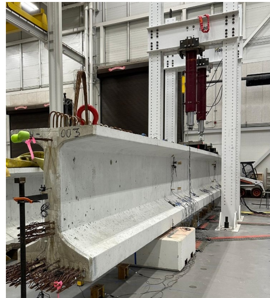
Figure 1. Shear Testing of Full-Scale Girder.
