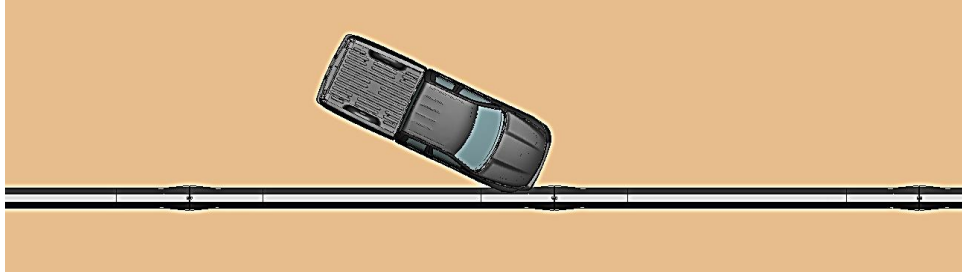
a. t = 0.17 s, event = pickup truck impacts barrier
