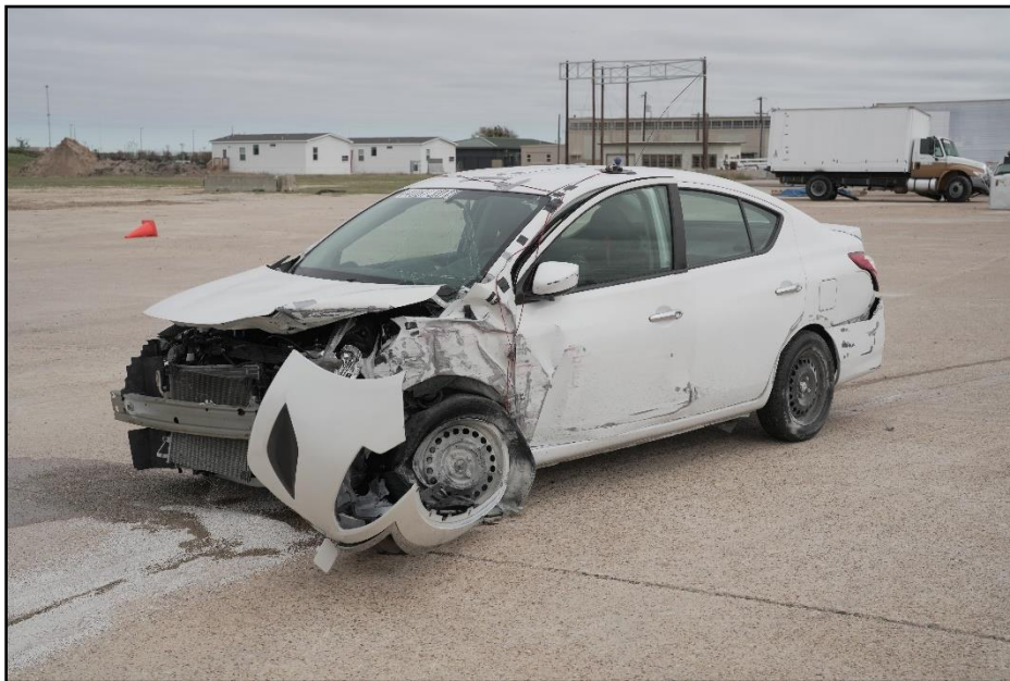
Figure 9.7. Impact Side of Test Vehicle after Test 440873-01-1.
