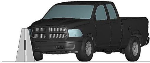
a. t = 0.18 s, event = pickup truck impacts barrier
