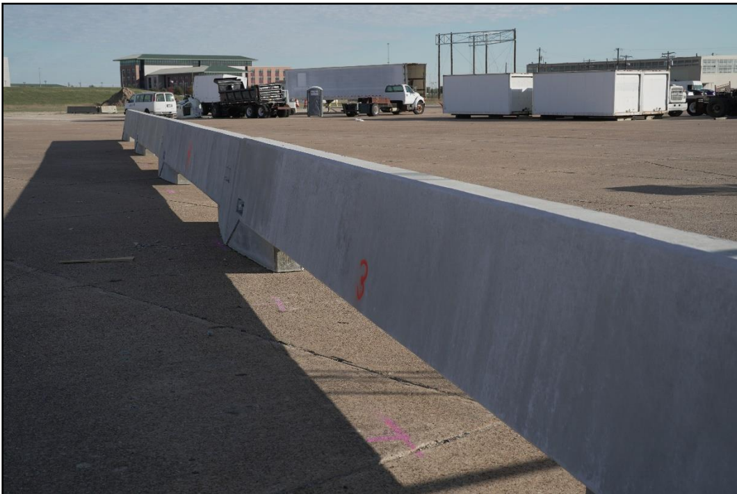
Figure 6.7. Field Side of the Large-Scupper Portable Concrete Barrier prior to Testing.
