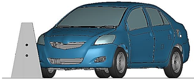
a. t = 0.19 s, event = front right tire contacts the barrier
