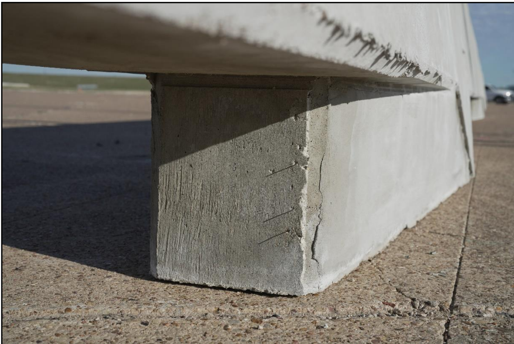
Figure 6.5. Close-Up of the End of the Scupper on the Large-Scupper Portable Concrete Barrier prior to Testing.
