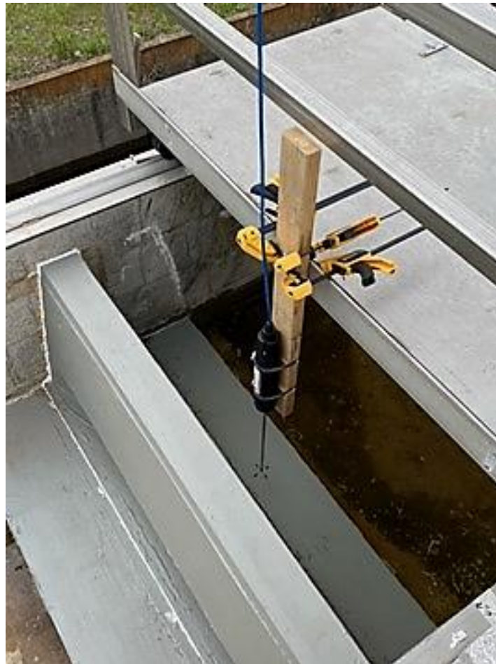
Figure 4.11. ADV Setup to Record Point Velocities Upstream of the Median Barrier.
