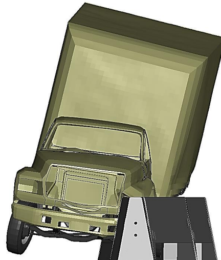
c. t = 0.94 s, event = front SUT tire stabilizes on the ground
