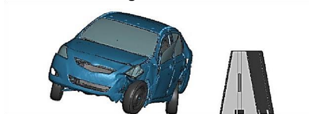
c. t = 0.91 s, event = rear right tire stabilizes on ground
