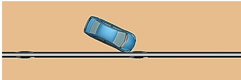
a. t = 0.17 s, event = passenger car strikes the barrier
