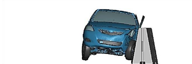
b. t = 0.23 s, event = rear right tire contacts the barrier, windowpane snags against the barrier
