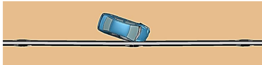
b. t = 0.23 s, event = passenger car contacts the joint
