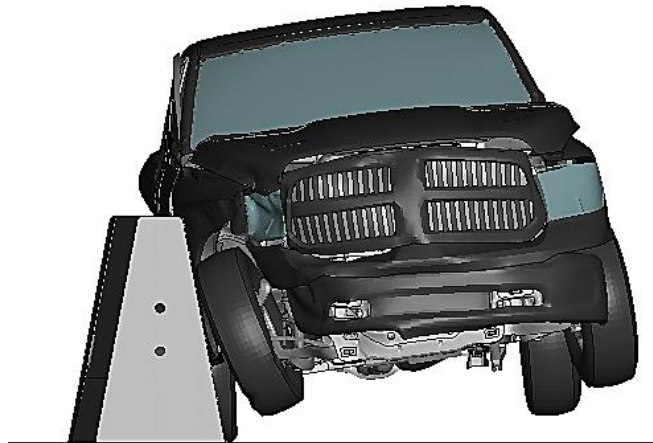
b. t = 0.35 s, event = rear right tire contacts the barrier
