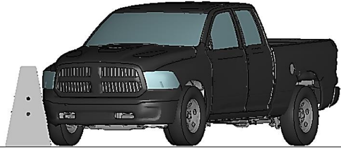
a. t = 0.17 s, event = front right tire contacts the barrier
