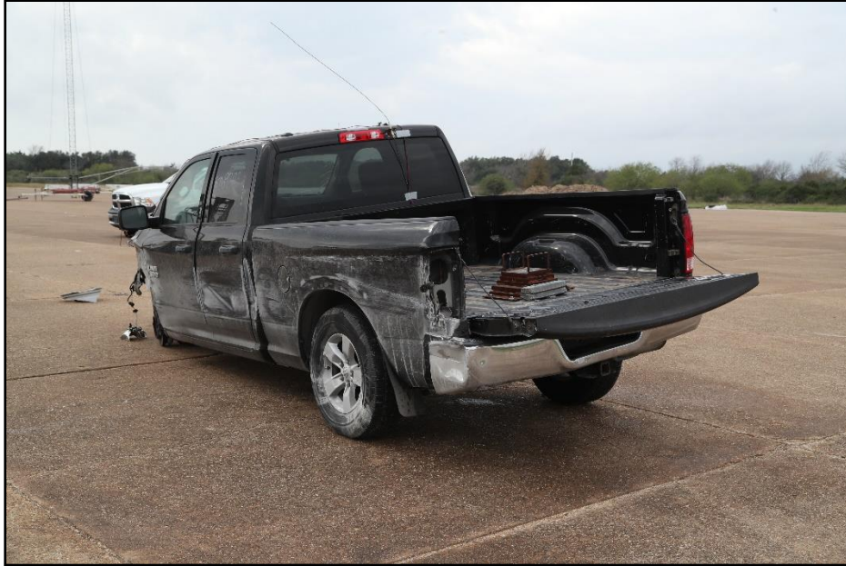
Figure 10.8. Rear Impact Side of Test Vehicle after Test 440873-01-2.
