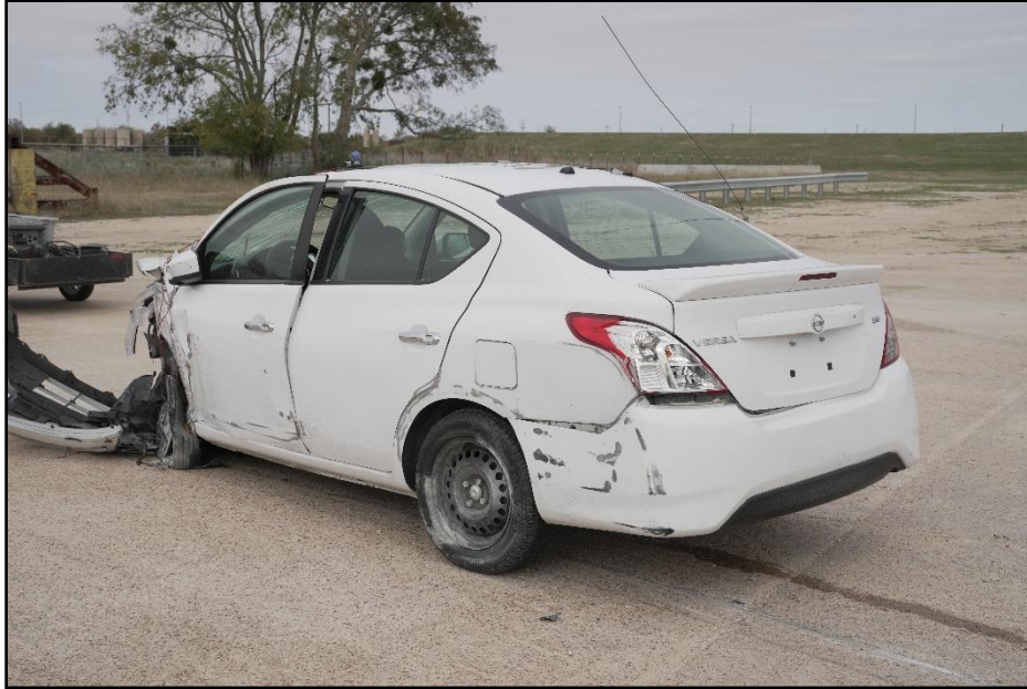
Figure 9.8. Rear Impact Side of Test Vehicle after Test 440873-01-1.
