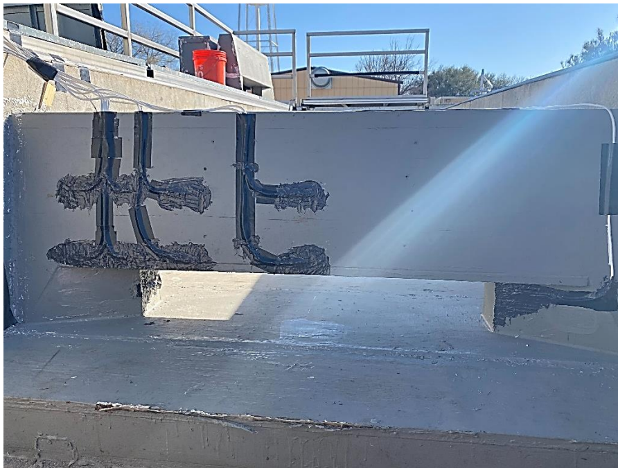
Figure 4.14. Strain Gage Setup after Environmental Coating.
