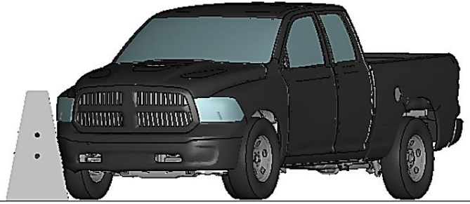
a. t = 0.17 s, event = front right tire contacts the barrier
