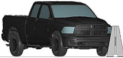
a. t = 0.10 s, event = front right tire contacts the barrier
