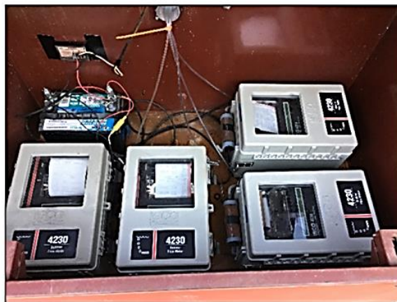
Figure 4.6. Bubble Flow Meters and Solar Panel Housing Unit (15).
