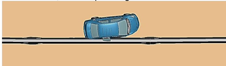
b. t = 0.33 s, event = passenger car completely engages the barrier
