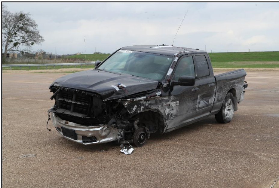
Figure 10.7. Impact Side of Test Vehicle after Test 440873-01-2.
