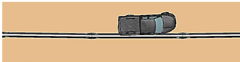
b. t = 0.34 s, event = pickup truck rear contacts the barrier
