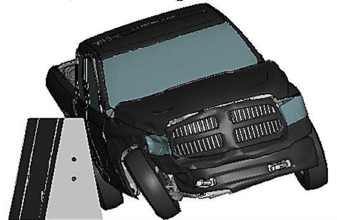
c. t = 0.57 s, event = front right tire touches the ground
