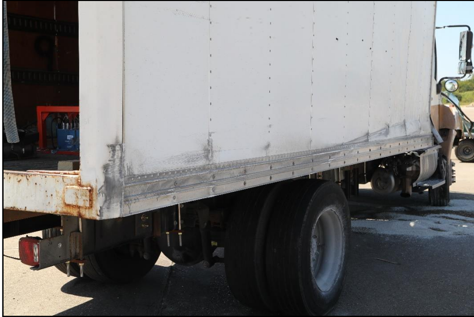
Figure 11.8. Rear Impact Side of Test Vehicle after Test 440873-01-3.
