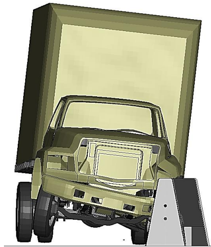
b. t = 0.53 s, event = SUT completely engages with the system
