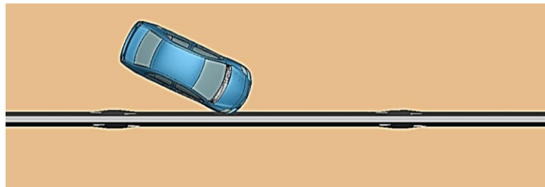
a. t = 0.17 s, event = passenger car strikes the barrier
