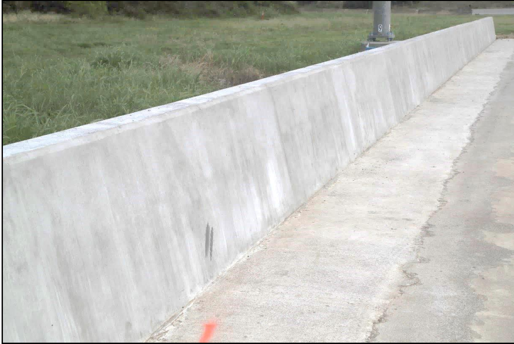
Figure 2.6. Overall View of the Luminaire Pole behind Single Slope Traffic Rail at Impact Prior to Testing.
