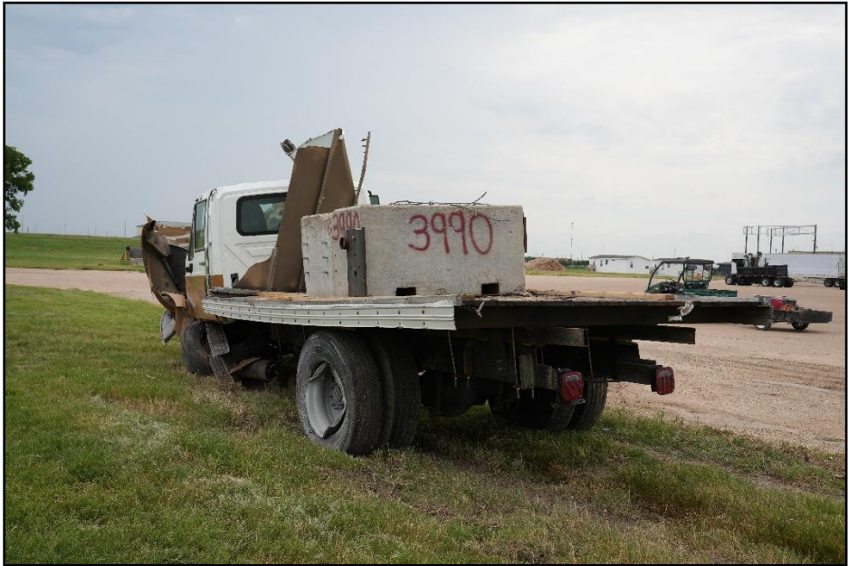
Figure 5.8. Rear Impact Side of Test Vehicle after Test 440863-03-1.
