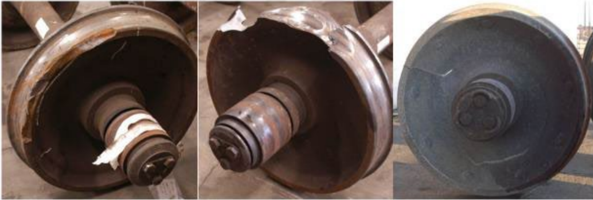
Figure 1. Example of Vertical Split Rim (left), Shattered Rim (center), and Thermal Crack (right) Failed Wheels [1]
