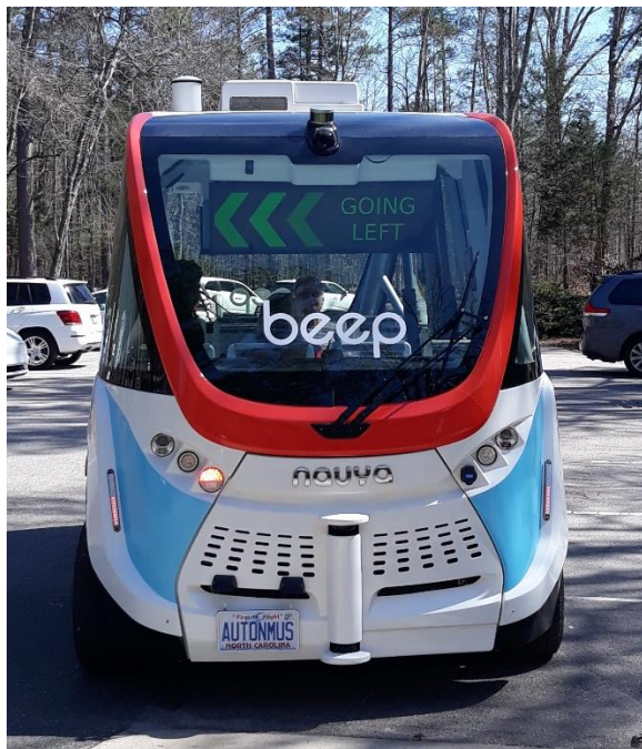
Figure 9. One of the shuttle's dynamic message boards indicates that the shuttle is "going left." Photo from the CASSI in Cary's Bond Park project. (Image courtesy of NCDOT)
