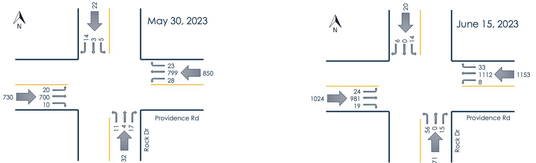
Figure B8. Day-to-Day Variation of Observed Volumes for C2, Intersection B, Map data © 2024 Google
