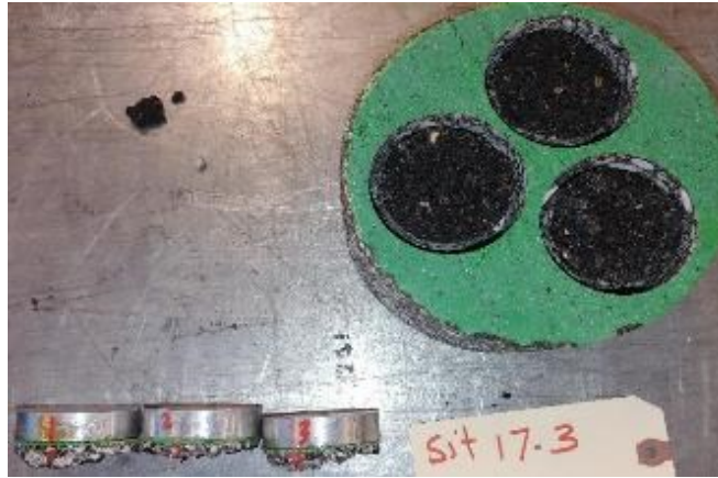
Figure 3-11. Substrate Failure near the Interface under Pull-Off Test.
