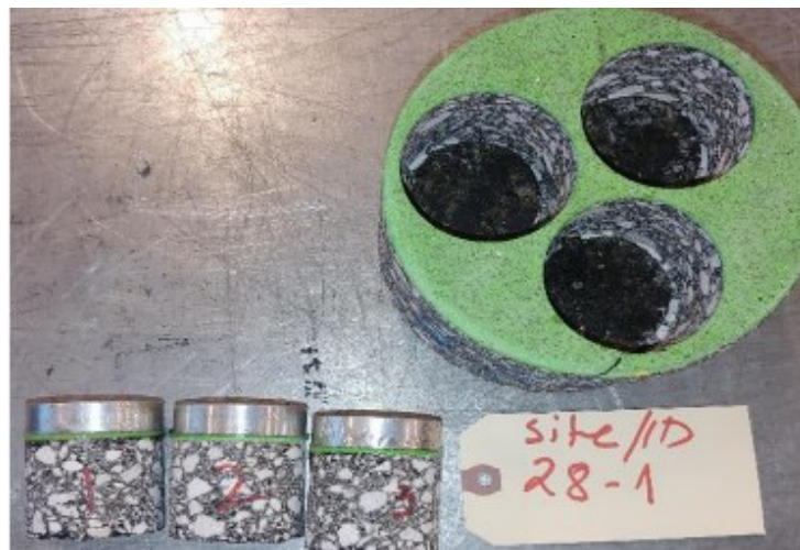
Figure B-8. Pull-Off Test for Specimen 28-1.
