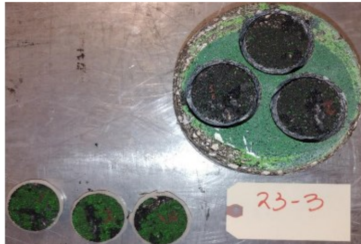
Figure B-3. Pull-Off Test for Specimen 23-3.
