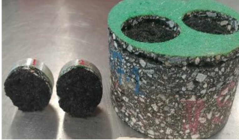
Figure B-15. Pull-Off Test for Specimen 7-1.
