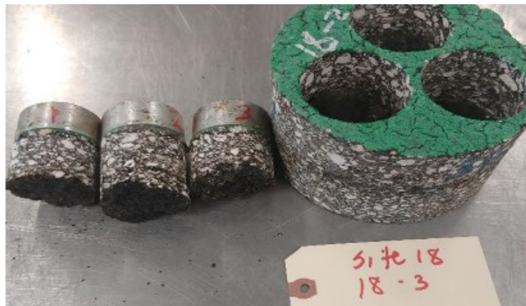
Figure B-14. Pull-Off Test for Specimen 18-3.
