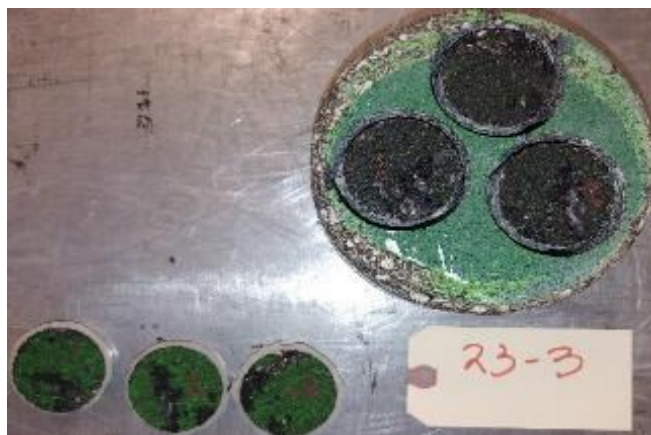
Figure 3-10. Clean Delamination under Pull-Off Test.
