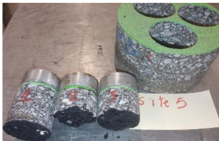
Figure B-4. Pull-Off Test for Specimen 5-1.
