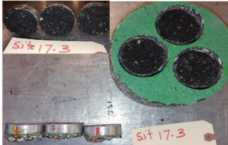
Figure B-7. Pull-Off Test for Specimen 17-3.
