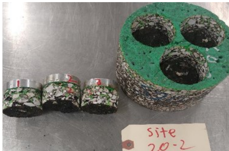
Figure B-9. Pull-Off Test for Specimen 20-2.
