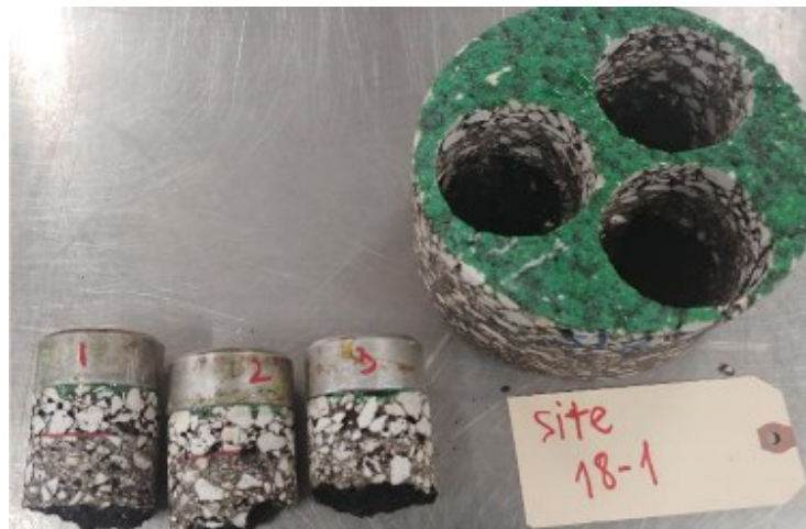
Figure B-12. Pull-Off Test for Specimen 18-1.
