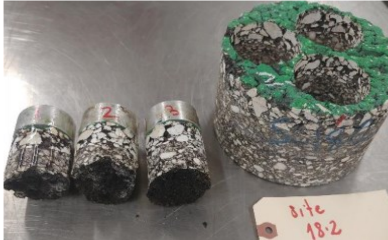
Figure B-13. Pull-Off Test for Specimen 18-2.
