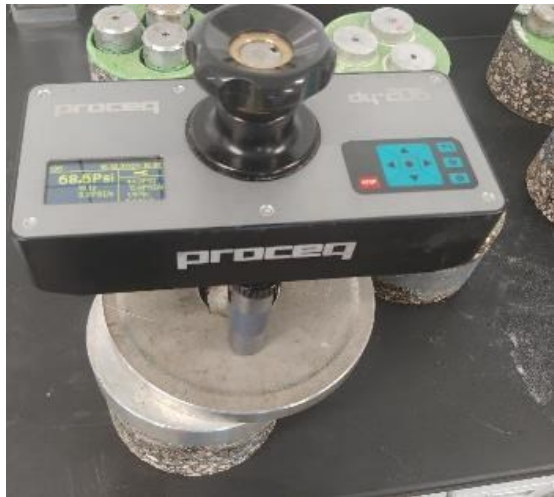
Figure 3-9. Pull-Off Test in Progress.
