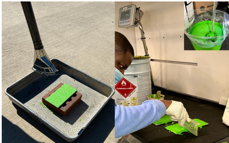
Figure 4-7. Preformed Thermoplastic and MMA Weathering Specimen Preparation.
