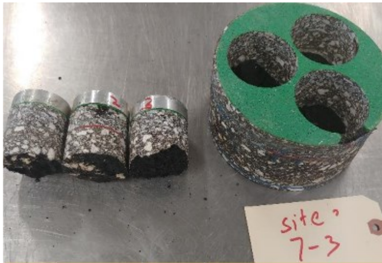
Figure B-16. Pull-Off Test for Specimen 7-3.
