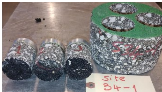
Figure B-6. Pull-Off Test for Specimen 34-1.
