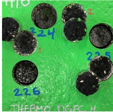
Figure 4-17. Pull-Off Test on Slabs after Freeze-Thaw.
