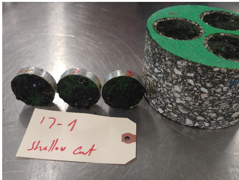
Figure B-19. Pull-Off Test for Specimen 17-1.
