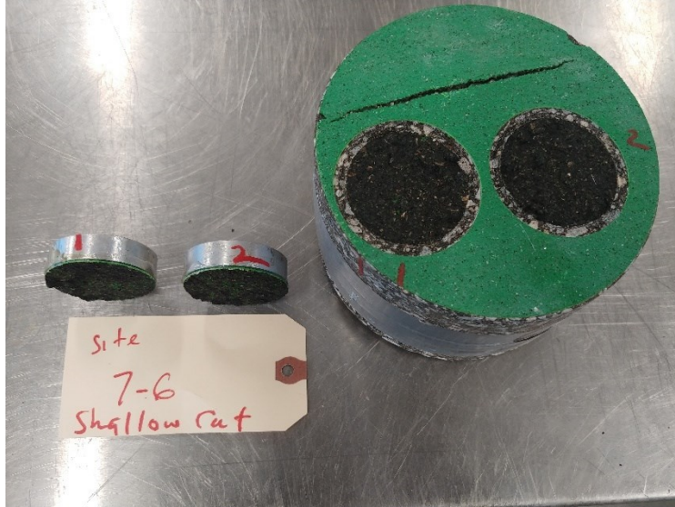
Figure B-18. Pull-Off Test for Specimen 7-6.
