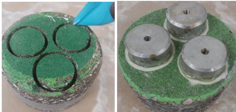
Figure 3-8. Gluing the Pull-Off Test Loading Discs.
