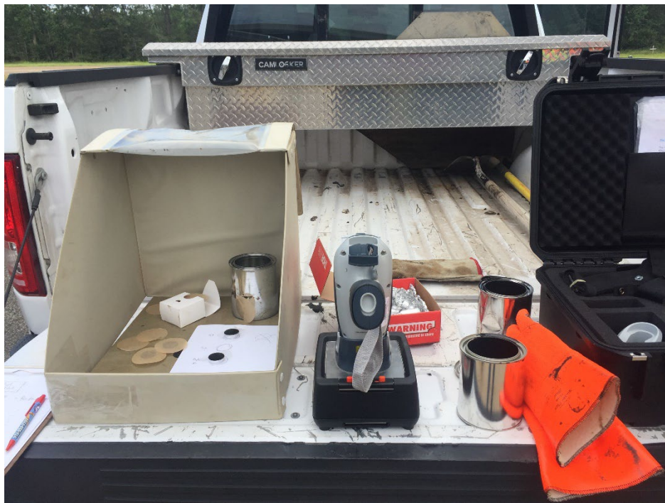
Figure 14. Portable XRF Field Testing Setup.
