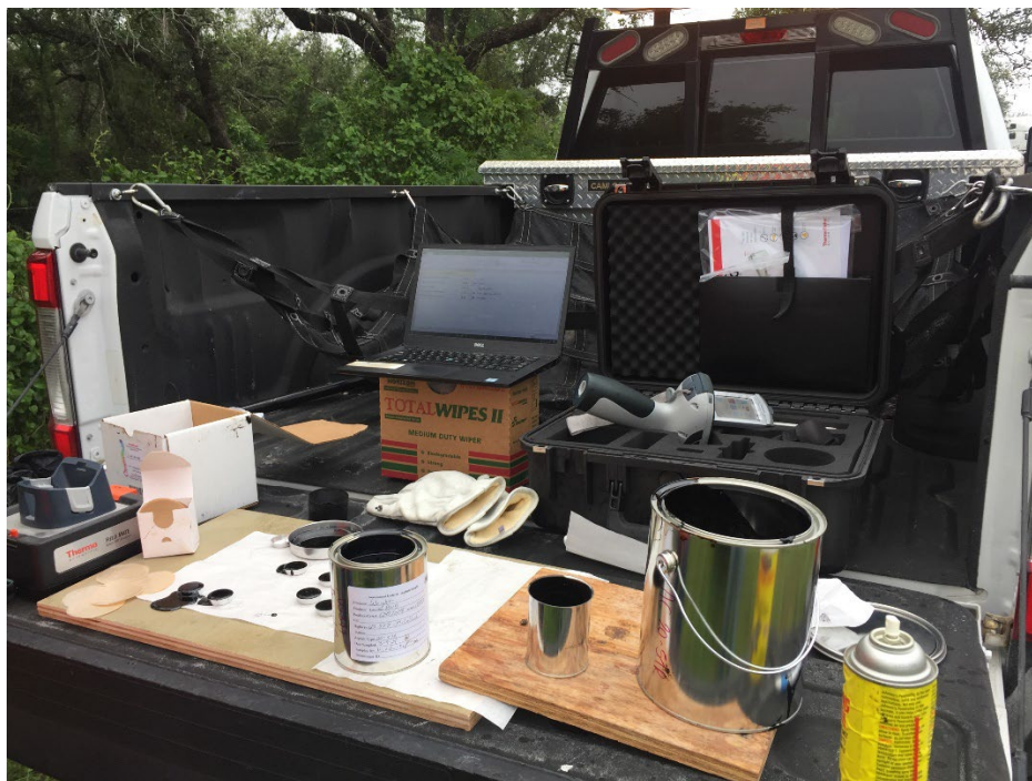
Figure 3. Portable XRF Field Testing Setup.
