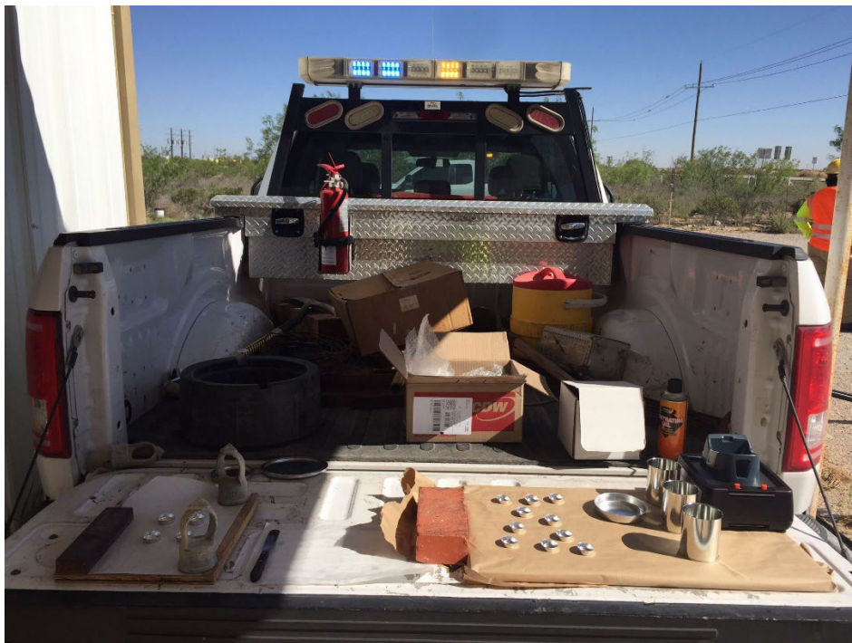
Figure 8. Portable XRF Field Testing Setup.
