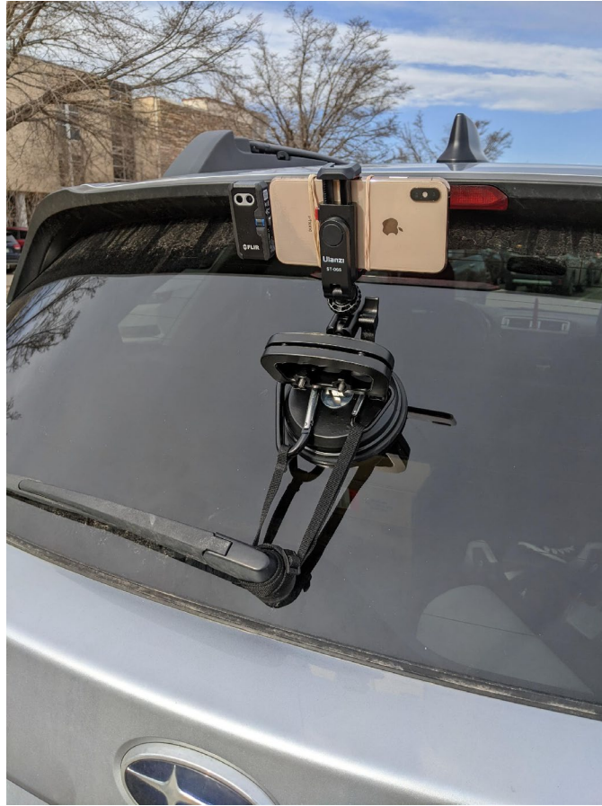
Figure 4.2 FLIR thermal camera setup
