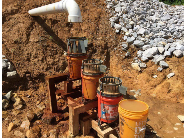
Figure 3-6. Sediment basin outlet flow divider bucket system used at the Morgan County site.
