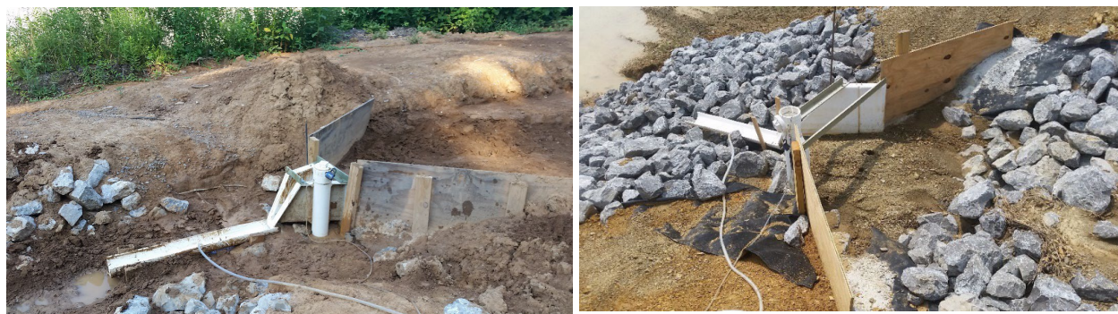
Figure 4-1. Sediment deposited at basin inlet H-flume for the Morgan County site (left) and the Knox County site (right).
