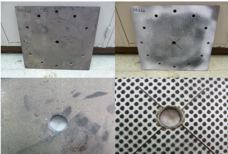
Figure 62: Fully penetrated tests (DB266 – 203.8 m/s) plate post-test. Clock wise: front view, rear view, rear view close up, front view close-up
