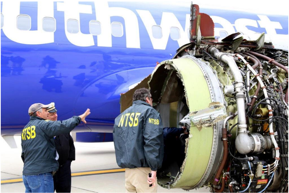
Figure 1: NTSB investigators examine the damaged Southwest Airlines engine on April 17 2018 [8]
