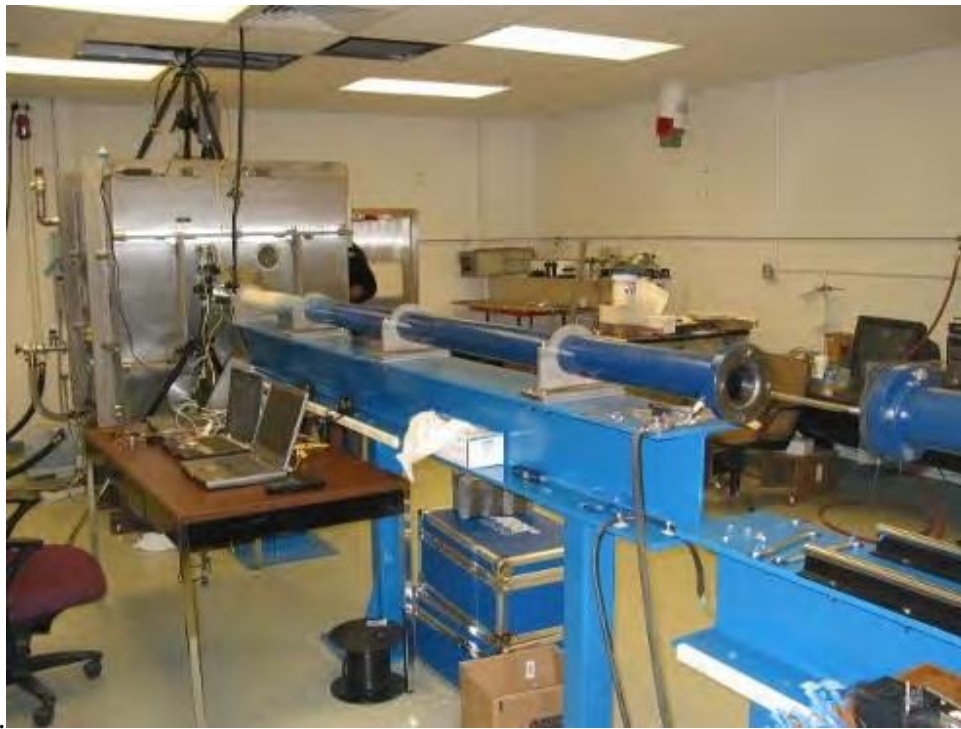
Figure 58: Large vacuum gas gun. Shown with 76.2mm (3 inch) diameter gun barrel [123]. (Image with 50.8 mm diameter barrel is not available.)
