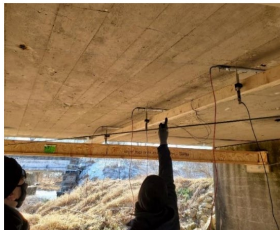
B. Photograph of the fixture with installed LVDT sensors
