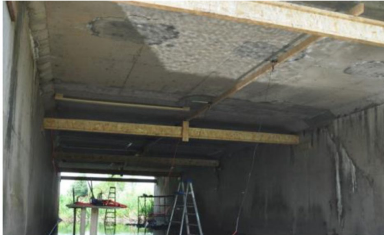
B. Wood fixture with installed LVDTs and strain gauge
