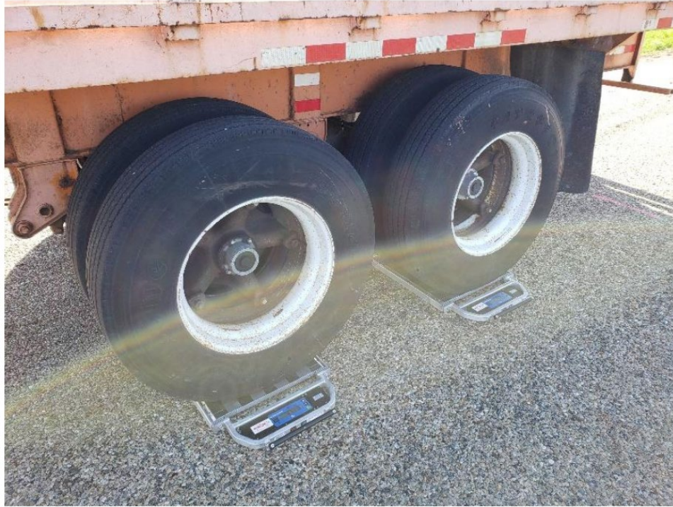
B. Movable scales used to measure axle loads during the proof load test
