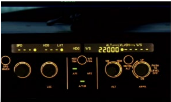
(h) Close-up view of flight control unit
