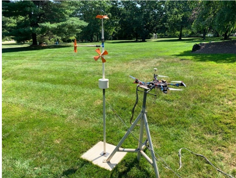
Figure 30. Instrumented Tarot 650 on sting balance with 3-axis anemometry stand
