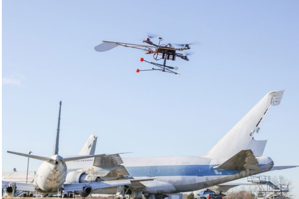
Figure 35. Quadcopter in transition behind B-737 exhaust flow
