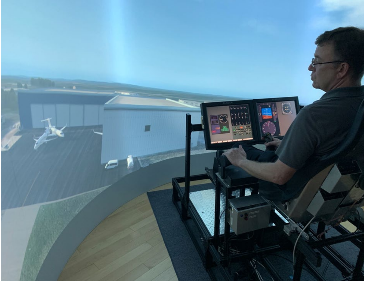
Figure 27. RCP display on left cockpit monitor in CDI's fixed base simulation lab
