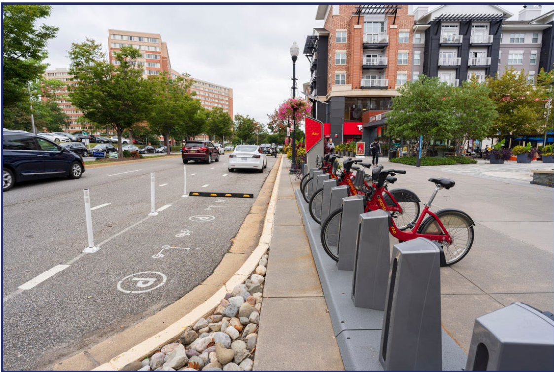
Figure 12. Photo. Example of curbside management applied in Washington, DC, to manage curb space for parking, micromobility, and other uses.
