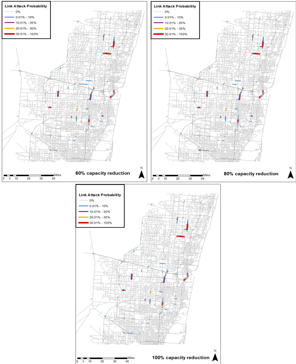
Figure 5. 17 Link's attack probability for 20 links per set under three different capacity reduction (60%, 80%, and 100%), Link attack selection: BC*
