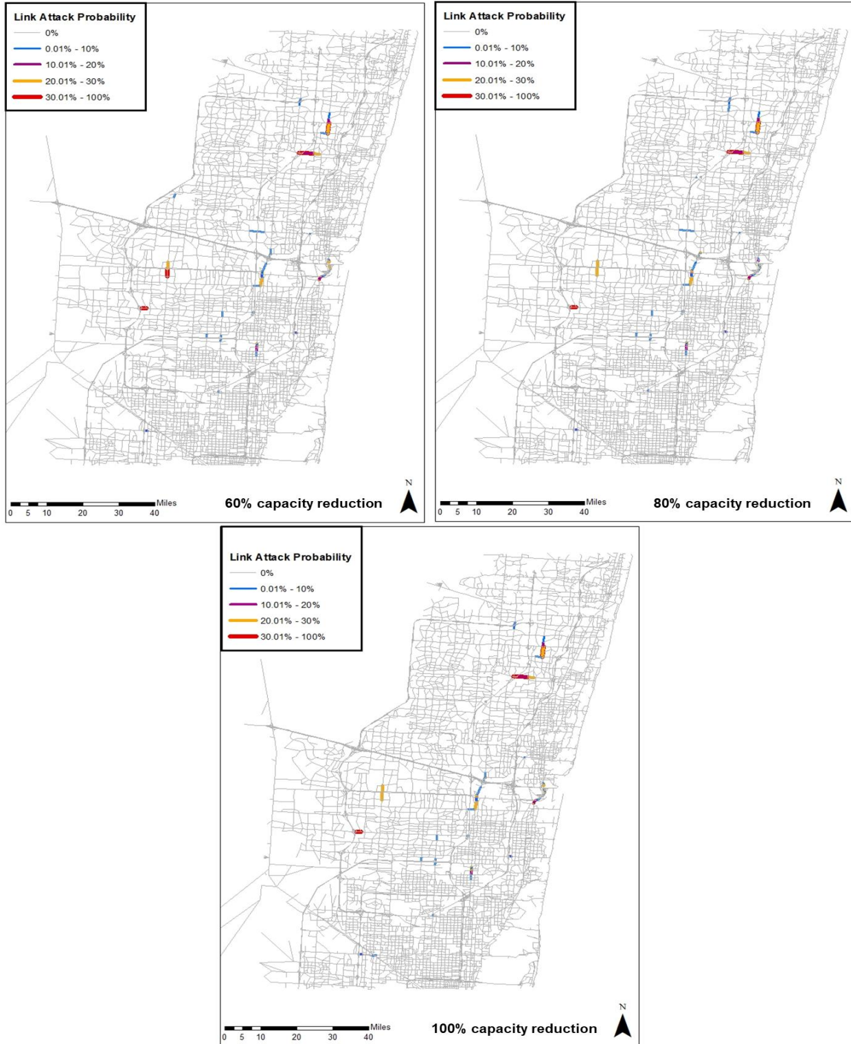
Figure 5. 16 Link's attack probability for 10 links per set under three different capacity reduction (60%, 80%, and 100%), Link attack selection: BC *
