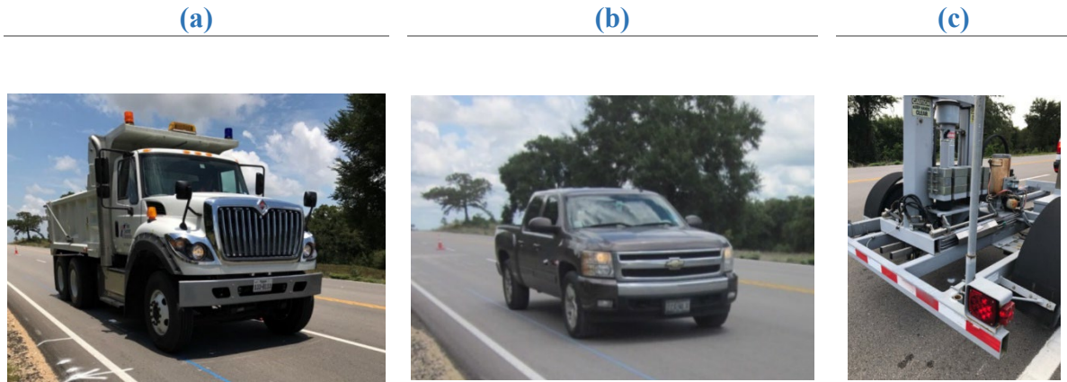
Figure 2.14. Controlled loading of instrumented geosynthetic-reinforced overlay sections along US77, Austin District: (a) heavy vehicle; (b) light vehicle; and (c) FWD.
