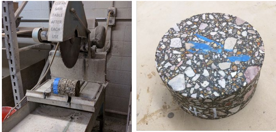
Figure 4.19. Photographs showing preparation of asphalt cores for characterization.
