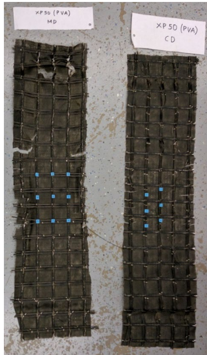
Figure 4.39. GS4 specimens in MD and CD after tensile test.
