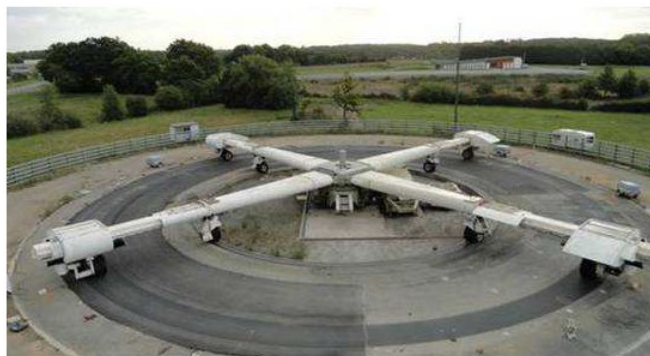
Figure 2.26. Photograph showing IFSTTAR fatigue test carrousel (IFSTTAR, 2012).
