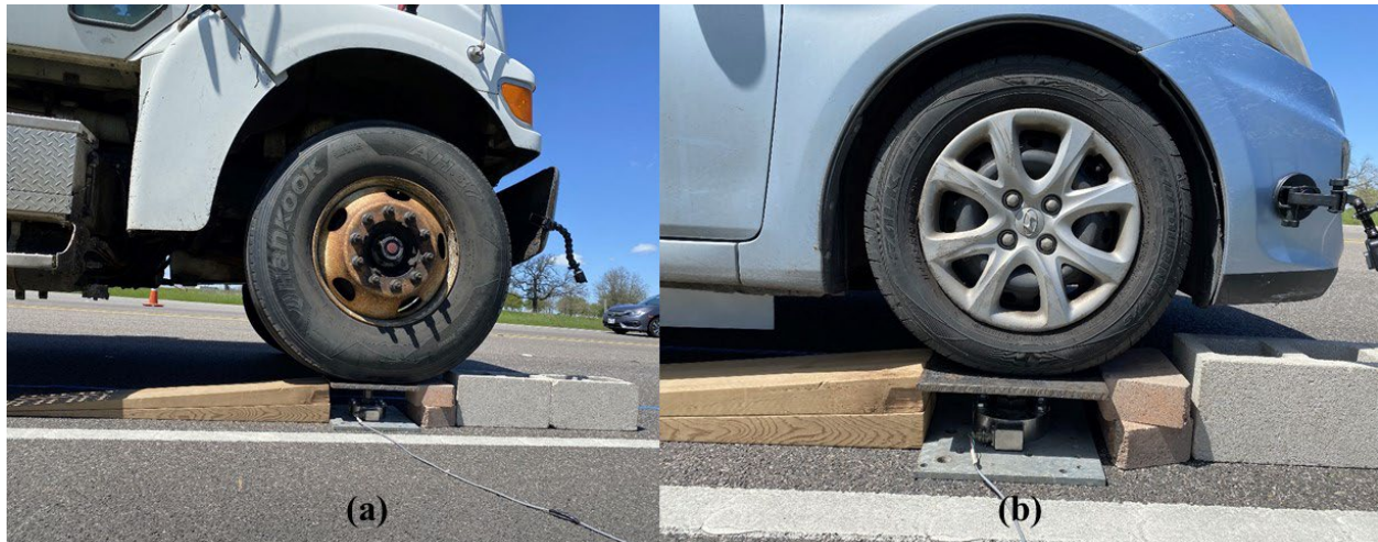
Figure 6.3. Custom scale used to weigh wheel load of: (a) heavy truck; and (b) light car.
