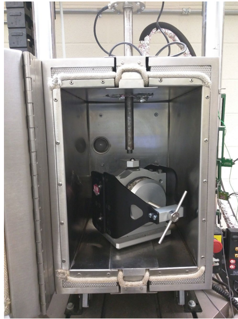
Figure 4.30. Asphalt-reinforcement interface shear test.
