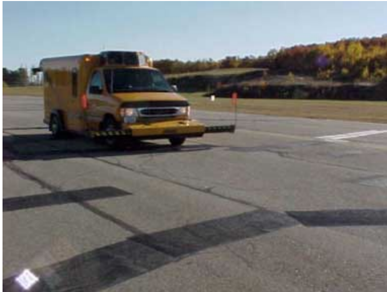
Figure 2.21. Photograph of Automatic Road Analyzer (ARAN) surveying test section (ME 01-3).
