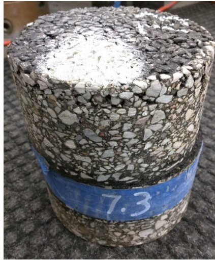
Figure 4.31. Pavement core from Section 7 after interface shear testing.
