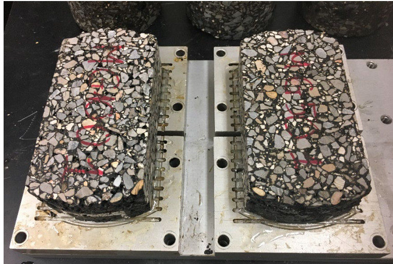
Figure 4.25. Asphalt specimens glued to base plates with spacer.
