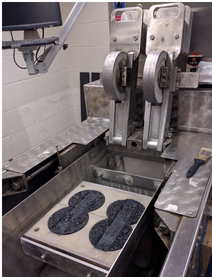
Figure 4.24. Hamburg wheel-tracking test device and asphalt specimen after test.
