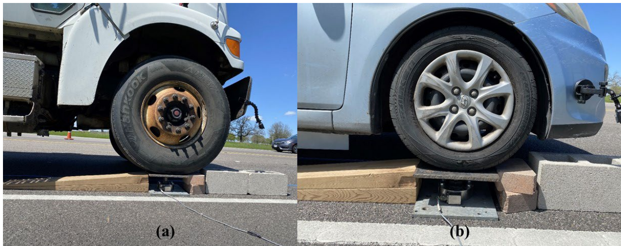
Figure 8.1. Custom scale used to weigh wheel load of: (a) heavy truck; and (b) light car.
