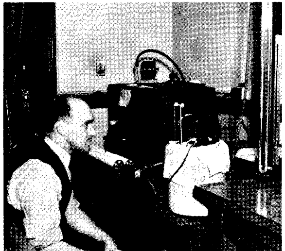
Figure 3.—Calibration chamber, during humidity calibration (Moist test). Recorder at right.
