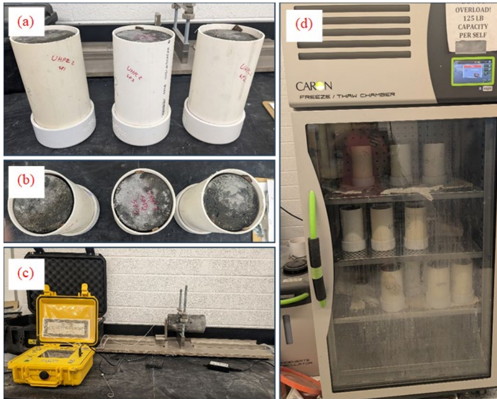
Figure 3.6 (a) and (b) Freeze-thaw durability test specimens, (c) Fundamental frequency and dynamic elastic modulus test setup, and (d) Freeze-thaw chamber with specimens
