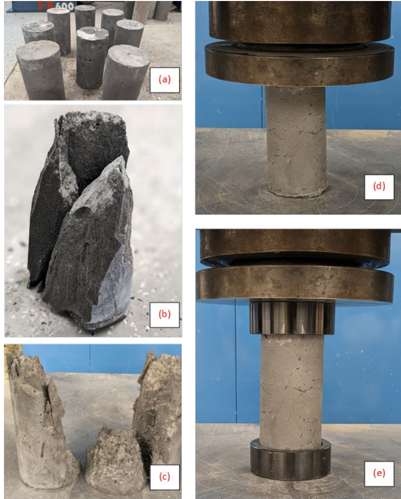
Figure 3.5 Compressive strength test: (a) Specimens, (b) Tested UHPC specimen with no fiber (c) Tested fiber-reinforced UHPC specimens, (c) Specimen with saw-cut end during test, and (d) Specimen with saw-cut end and neoprene pad during test
