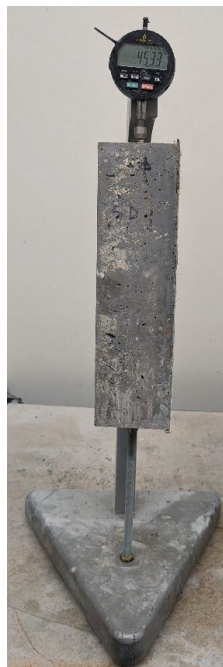
Figure 3.8 Drying shrinkage test setup
