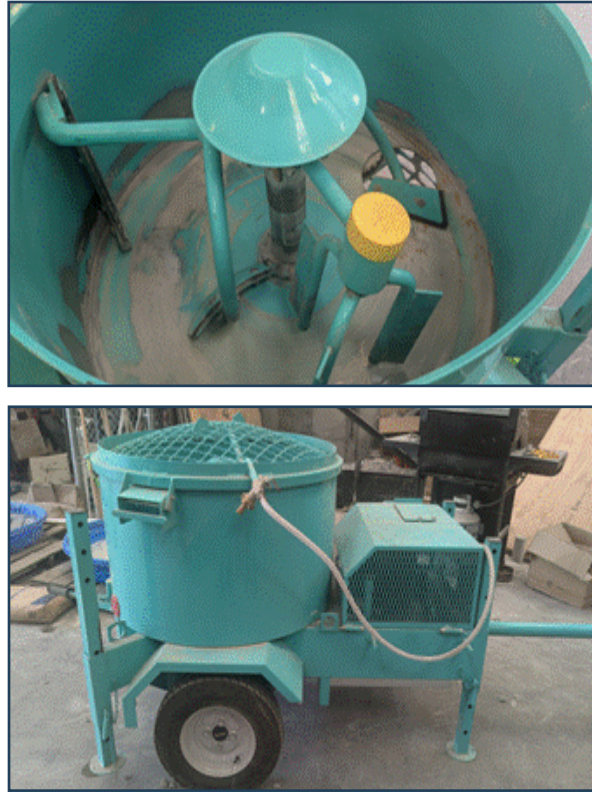
Figure 4.6 IMER 360 Plus mixer used to cast a large batch of UHPC
