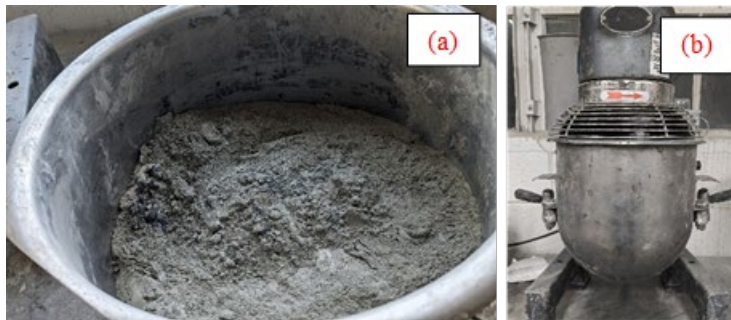
Figure 3.3 (a) Dry ingredients in mixing bowl, (b) tabletop mixing machine
