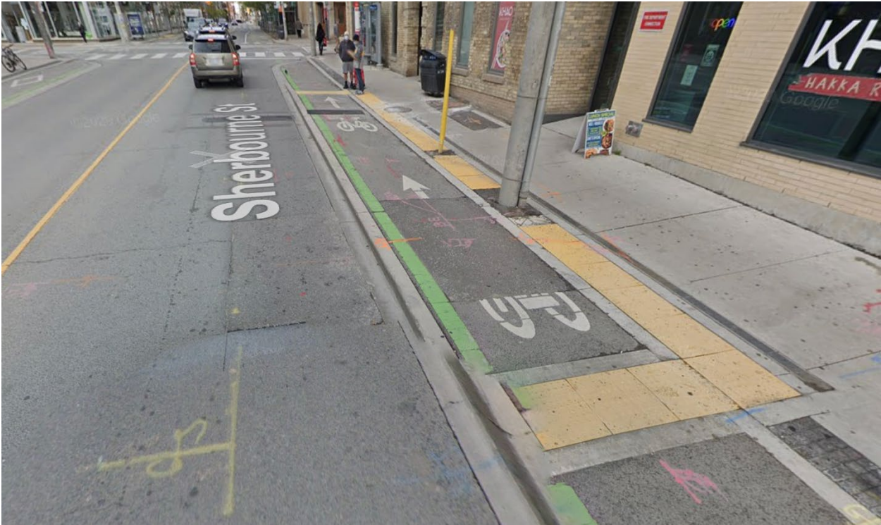
Figure 12 Cycle track bus stop with no additional boarding area. Toronto, ON, Sherbourne Street (Source: Google Street View)
