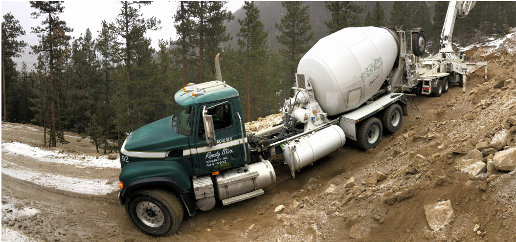
Figure 7: Concrete Mixer with Driver-Side Mounted Water Tank
