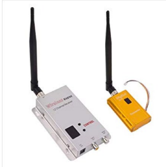
Figure 32. 1.2 GHz video transmitter and receiver
