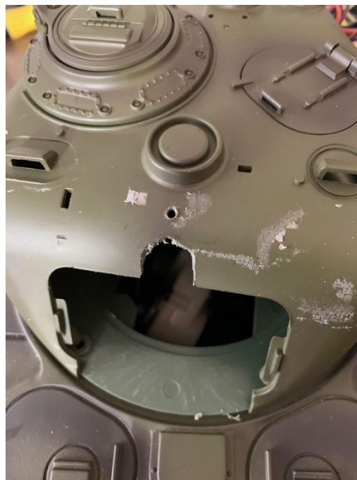
Figure 76 1/2-inch hole drilled for Camera 1 mounting
