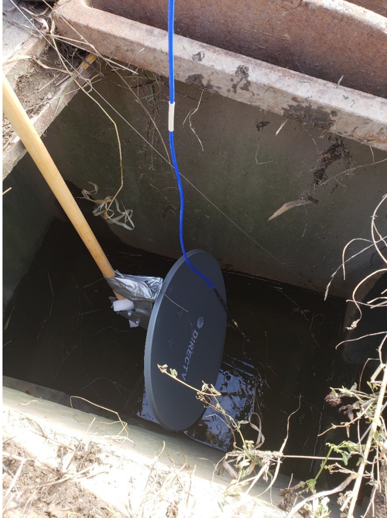
Figure 63 Antenna on extension cable and reflector dish inserted through drop inlet utility hole into telemetry beam line projecting from culvert
