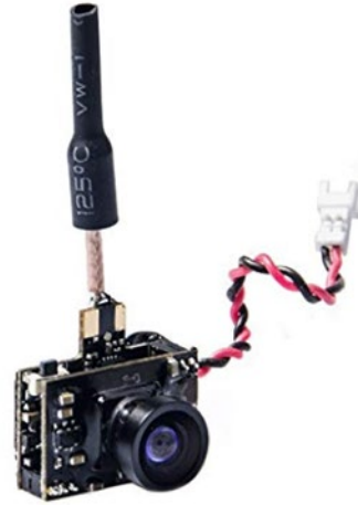
Figure 35. Camera with integrated 5.8 GHz transmitter
