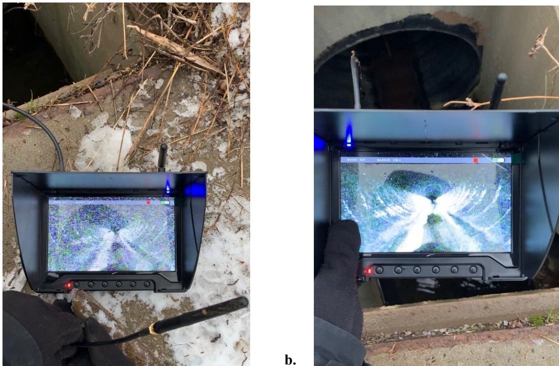
Figure 51 Telemetry Option Test 4 results comparison between antenna in and out of DI: a. Antenna out of DI, b. Antenna in DI
