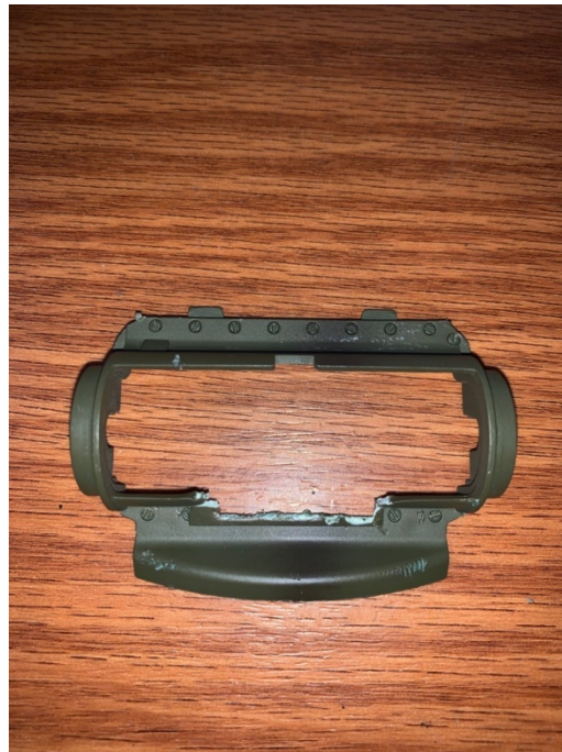
Figure 81 Camera 2 cover with cut made for camera
