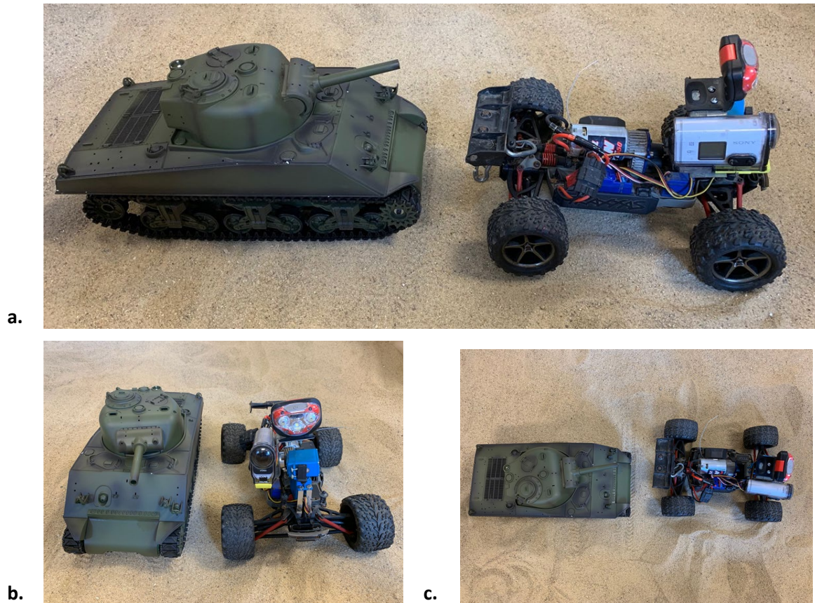
Figure 6 HIVE 1.0 v. HIVE 2.0: a. Side view, b. Front view, c. Top view
