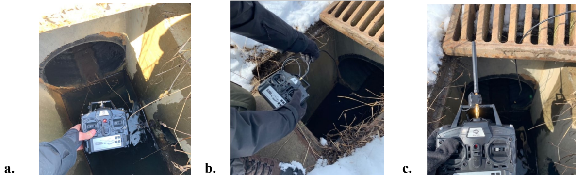
Figure 59 Telemetry Option Test 7 HIVE 2.0 controller modification effects on range: a. Unmodified controller, b. Controller with extension cable, and c. Controller with amplifier
