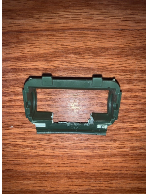
Figure 80 Camera 2 cover with plastic connectors removed
