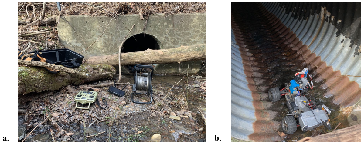
Figure 40. Telemetry Option Test 2 setup, HIVE 1.0 instrumented with 1.2 and 5.8 GHz video systems placed inside Culvert 64099 entrance for reception test at the other end
