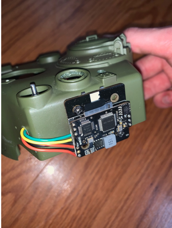
Figure 84 Transmitter screwed to back of turret
