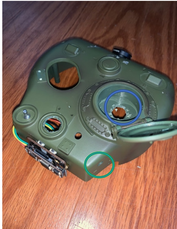
Figure 86 Holes drilled for antenna
