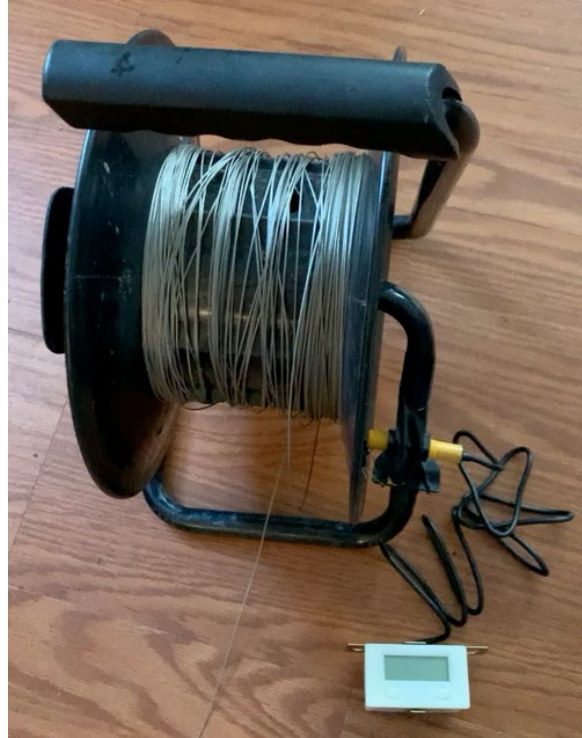
Figure 20 Retrieval wire spool with magnetic revolution counter
