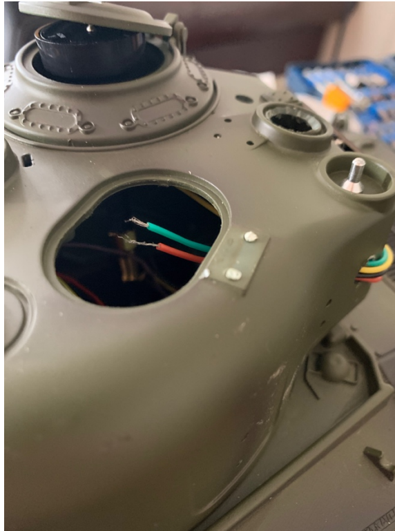
Figure 87 Hatch door removed and partially protruding antenna mount
