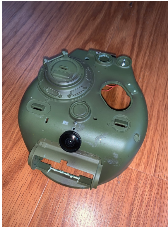
Figure 82 Camera 2 cover bonded to turret shell
