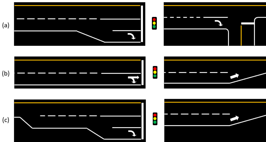
Figure 3-1 Special lane drop configurations: (a) trap lane, (b) through/right lane, (c) ATL.
