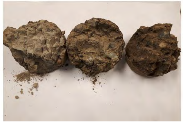
Figure 3.16. The moisture content of 2%, 4%, and 6 % specimens after breaking the specimens.
