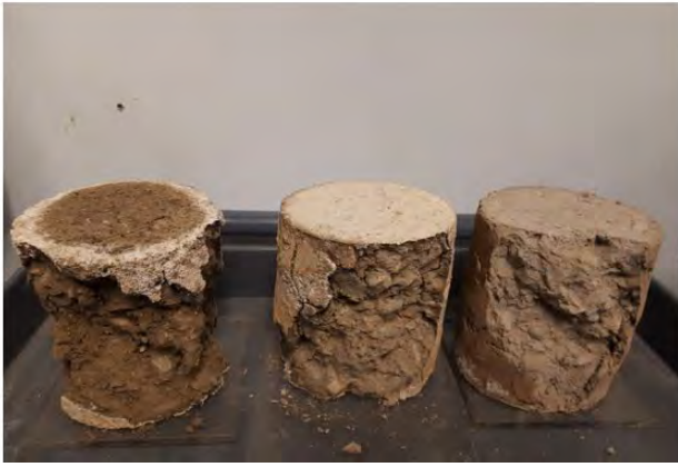
Figure 3.16. The moisture content of 2%, 4%, and 6 % specimens after breaking the specimens.
