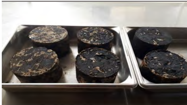
Figure 2.16. Photo of the prepared asphalt emulsion specimens
