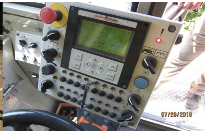
(d) Control panel inside Wirth 2500 S cab showing fluid injection and grinding controls
