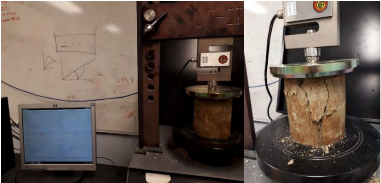
Figure 2.13: Unconfined compressive strength testing of 4% cement stabilized specimen
