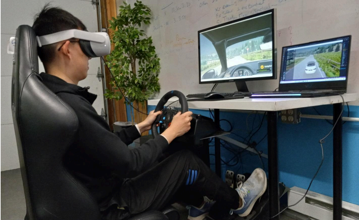
Fig. 5. Simulator demonstration: left monitor shows Carla server first person driver's seat view; right monitor shows the Carla client third person tracking view.
