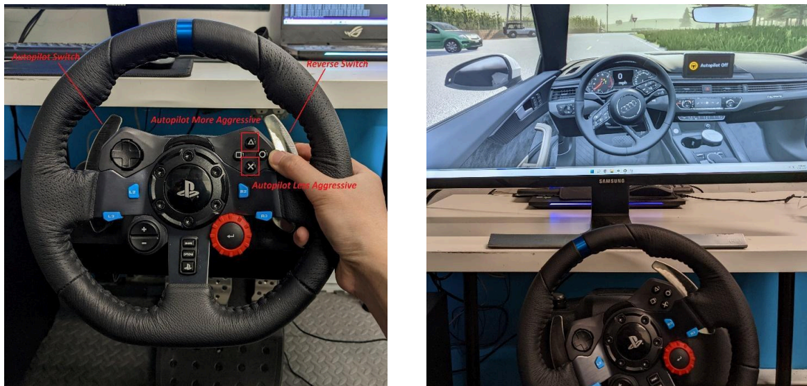
Fig. 1. Logitech G29 wheel explanation. Left: functions for buttons and switches. Right: physical and simulation wheel correspondence.
