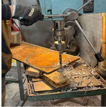
Figure C.1 Preparing the compaction plate for the compressibility test with soil-TDA Type A mixtures
