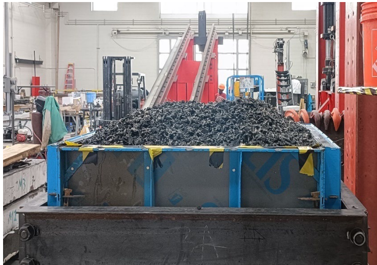
Figure 4.8 Filling the upper shear box with TDA Type A
