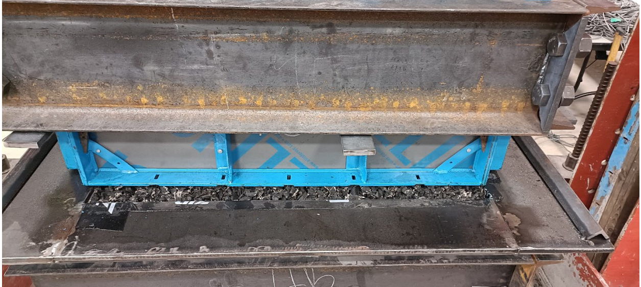
Figure B.7 The TDA Type A after shearing
