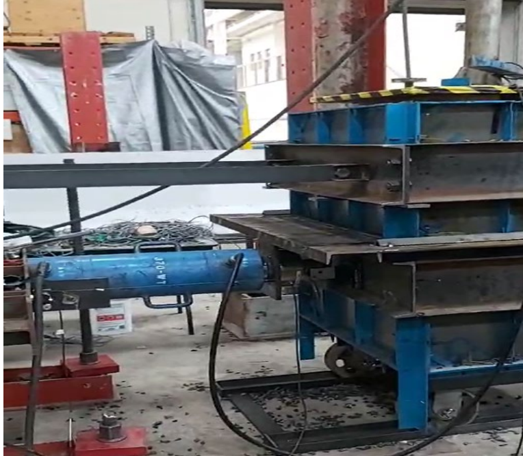
Figure B.5 Getting the test ready before running the direct shear test
