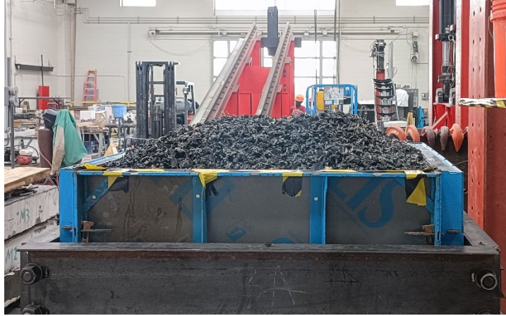
Figure B.3 Filling the shear box with TDA Type A
