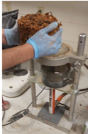
Figure A.12 Extracting the soil-TDA sample from the mold
