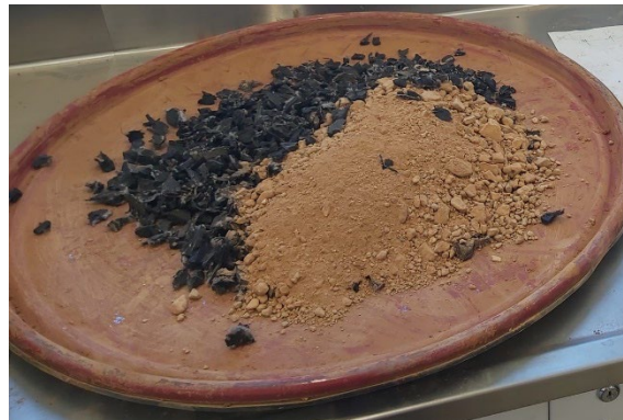
Figure A.10 Mixing the soil with TDA Type A to determine the optimum water content and the max dry density
