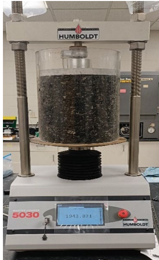
Figure C.3 TDA Type A compressibility test
