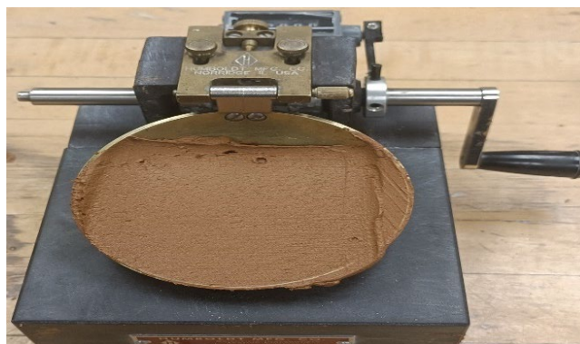
Figure A.15 Determining the liquid limit for the soil
