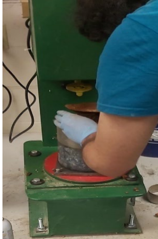
Figure A.7 Proctor test for the soil to determine the optimum water content and the max dry density
