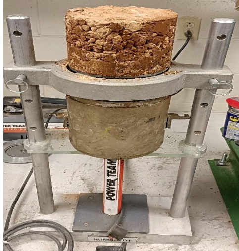
Figure A.9 Extracting the soil sample from the mold
