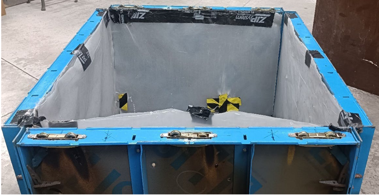
Figure 4.4 The upper shear box after installing the outstanding rollers
