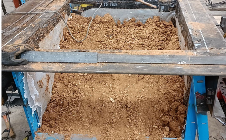
Figure B.11 Getting the soil outside the lower box
