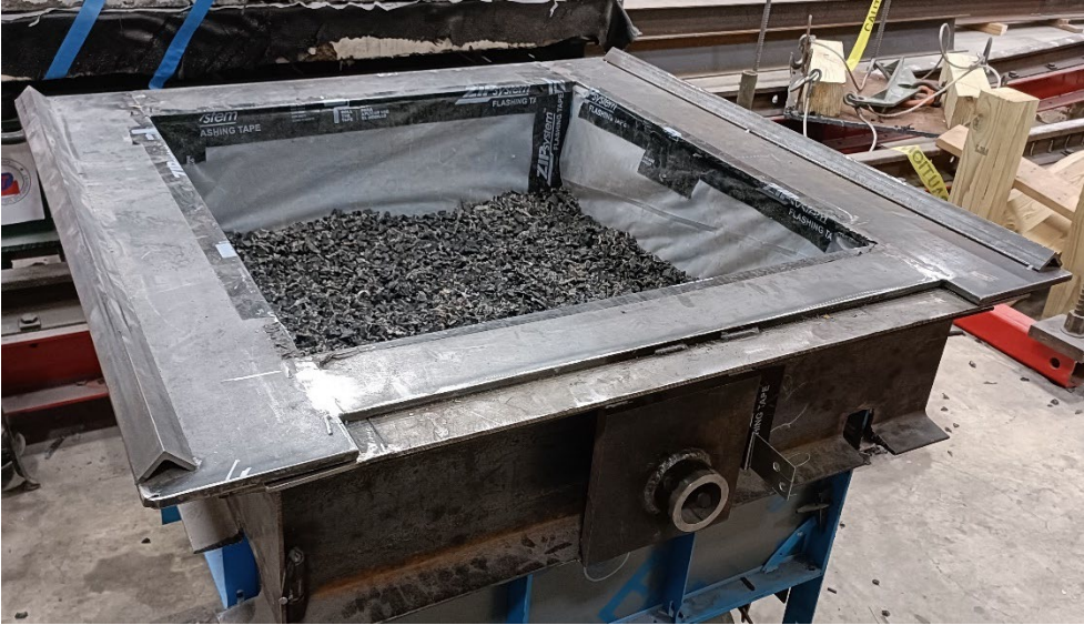
Figure 4.5 Filling the bottom shear box with TDA Type A
