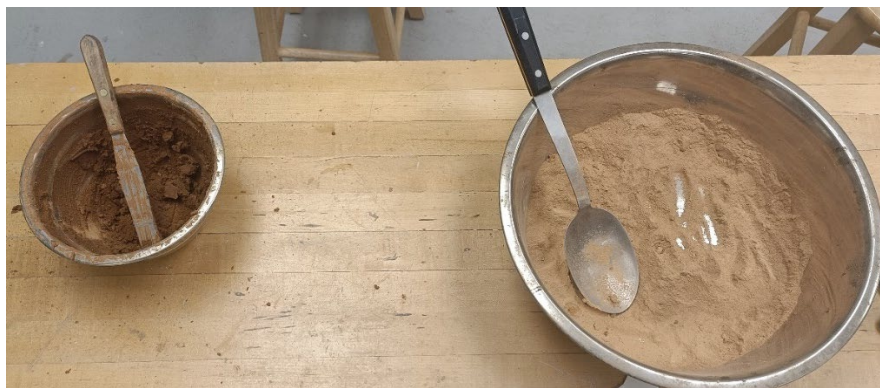
Figure A.14 Mixing the soil to get the Atterberg limits
