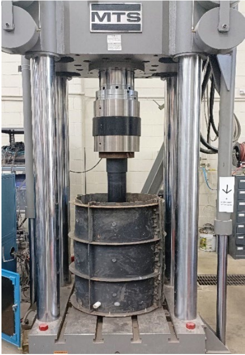
Figure D.1 Running the compressibility test with soil-TDA Type B mixtures
