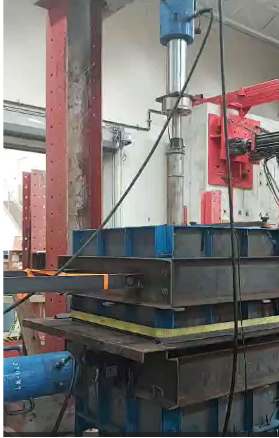
Figure 4.9 Placing the upper box in its place preparing for the direct shear test
