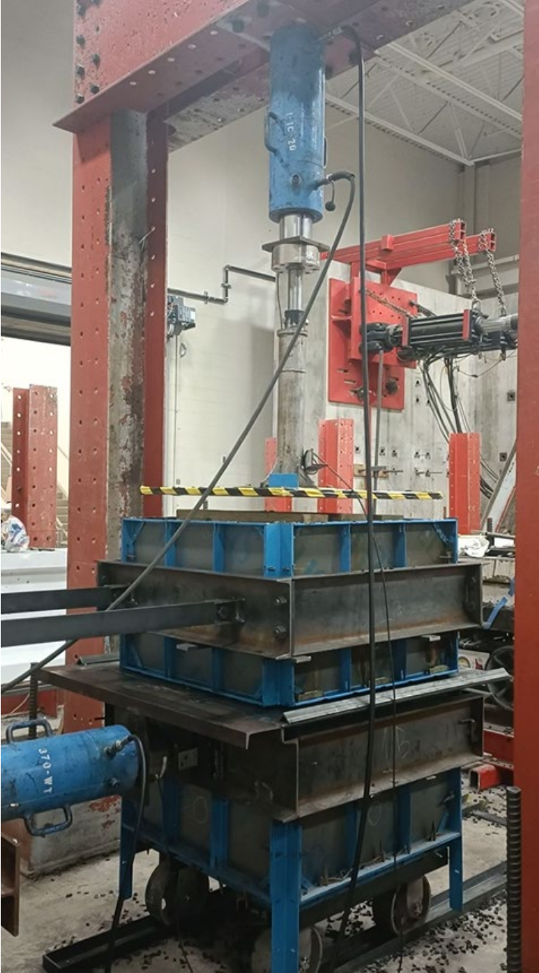
Figure 4.1 Large-scale direct shear test device
