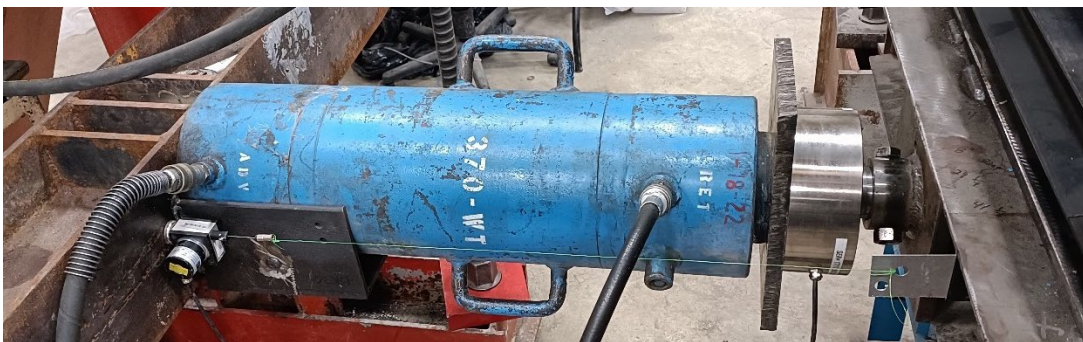
Figure B.4 Attaching the string pot to measure the horizontal displacement before the direct shear test
