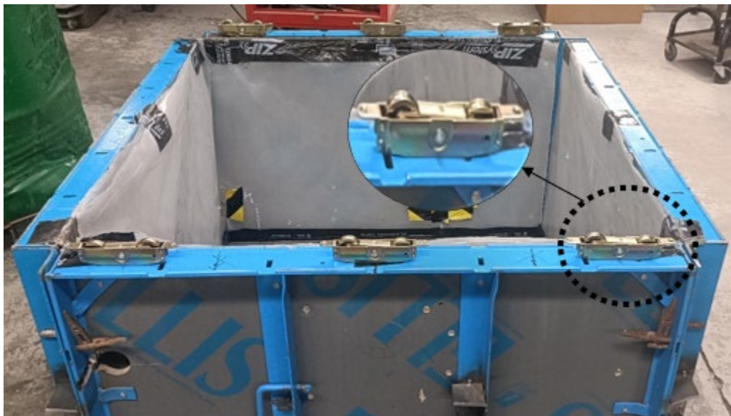
Figure 4.3 The upper shear box before installing the outstanding rollers
