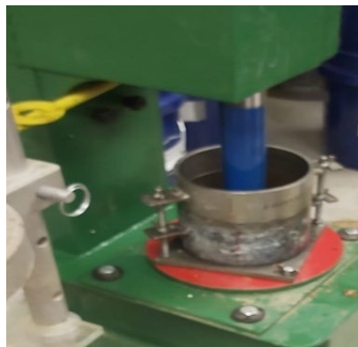
Figure A.8 Compaction of the soil sample in three layers
