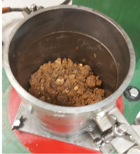
Figure A.11 Compaction of the soil-TDA sample in three layers
