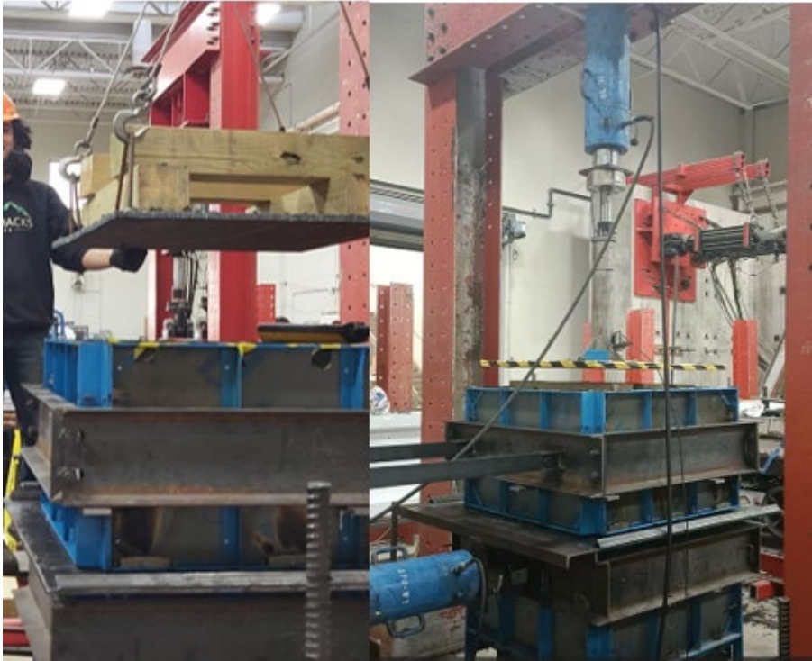
Figure 4.6 Compacting the different samples before the test
