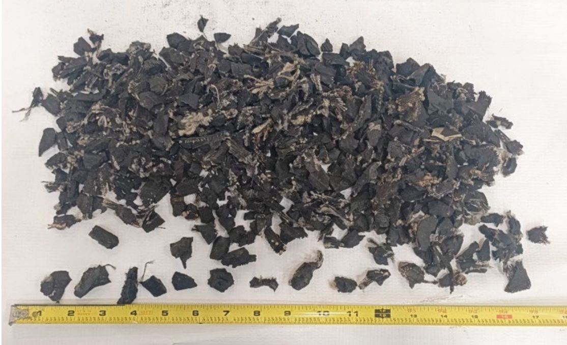
Figure 3.1 The Type A TDA sample used in this study
