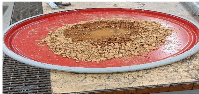
Figure A.6 Mixing the soil with water to determine the optimum water content and the maximum dry density
