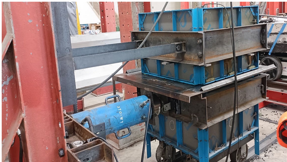
Figure B.6 Running the direct shear test
