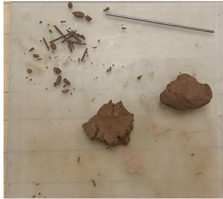
Figure A.16 Determining the plastic limit for the soil
