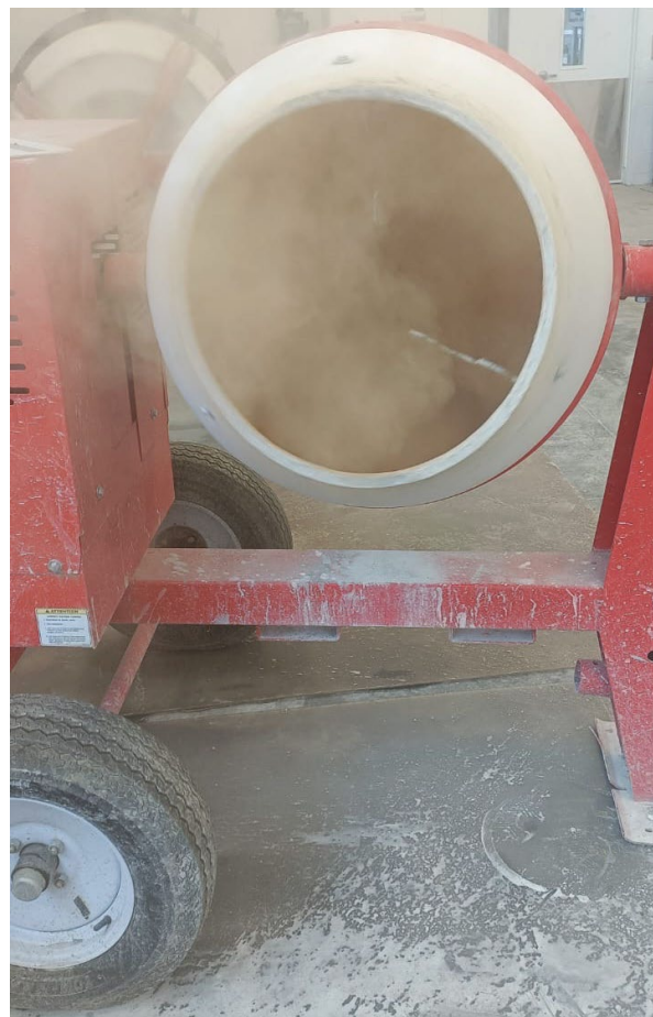
Figure A.4 Crushing the soil inside the mixer
