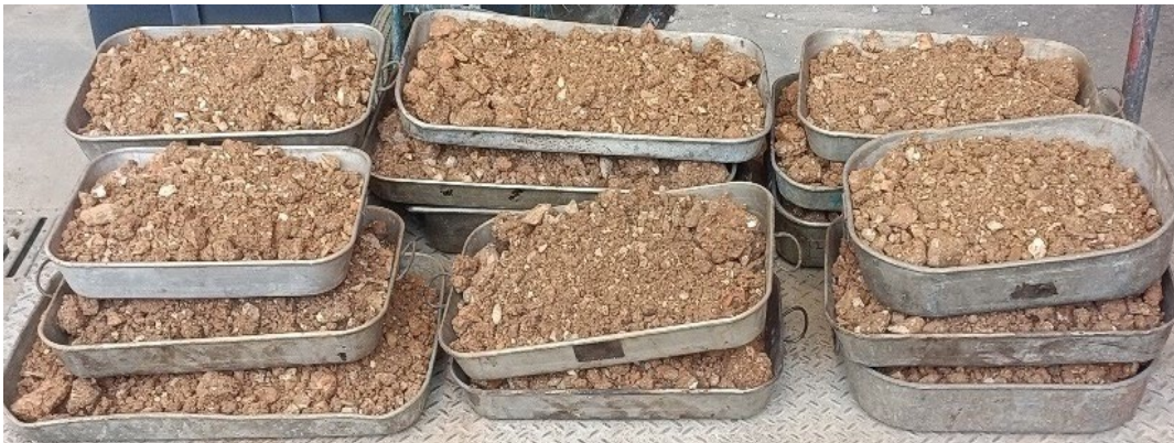
Figure A.2 Preparing the soil before putting it inside the oven to get it fully dry
