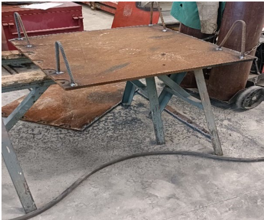
Figure B.2 Preparing the compaction plate used to compact the samples inside the shear box before testing
