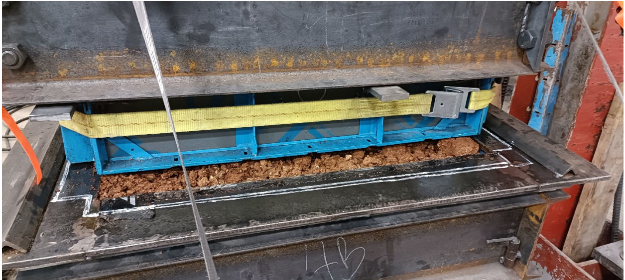
Figure B.8 The soil after shearing
