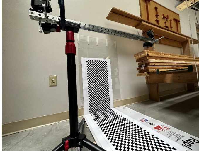
Figure 2.3 3D calibration target setup for dual stereo pairs calibration with the camera rig suspended above the target
