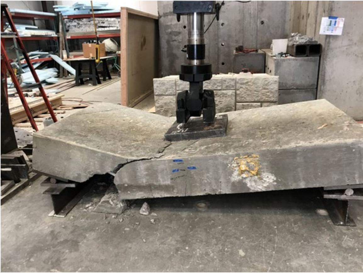
Figure 5.20 GFRP Catastrophic Failure
