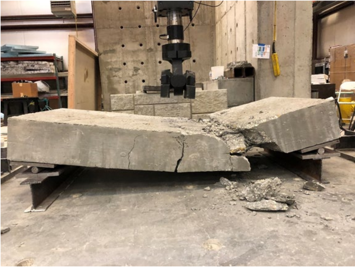
Figure 5.10 Panel with Steel Reinforcement Catastrophic Failure
