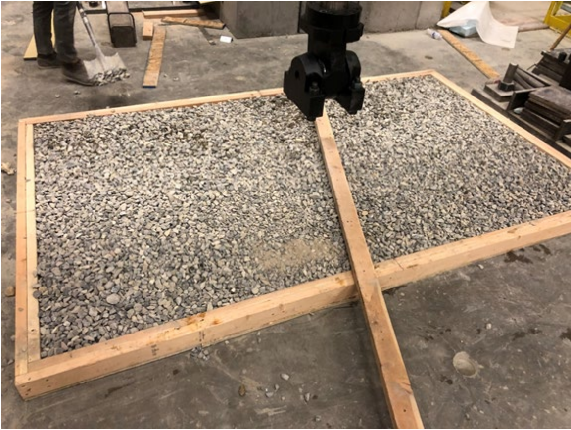
Figure 3.4 Gravel Containment Box
