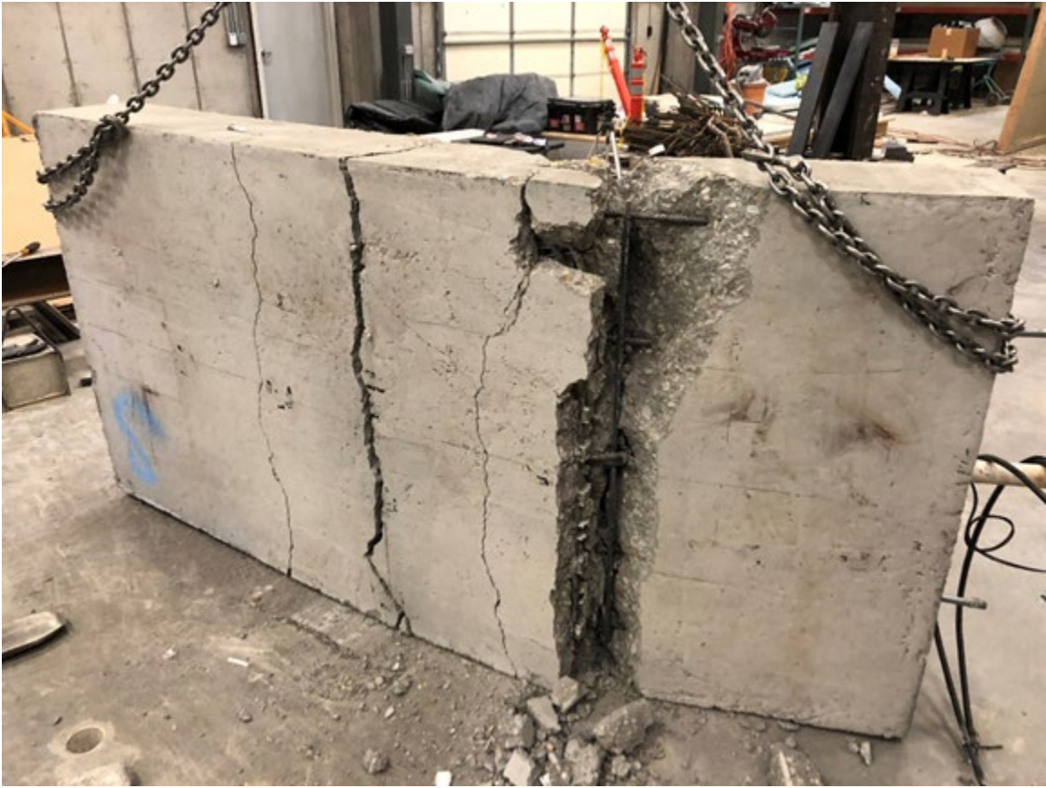
Figure 5.12 Face of Steel Reinforced Slab After Failure
