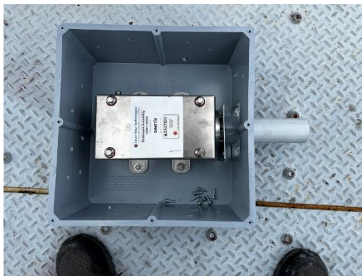
(a) View of NEMA 4X laser located within one of the non-metallic enclosures, prior to installation
