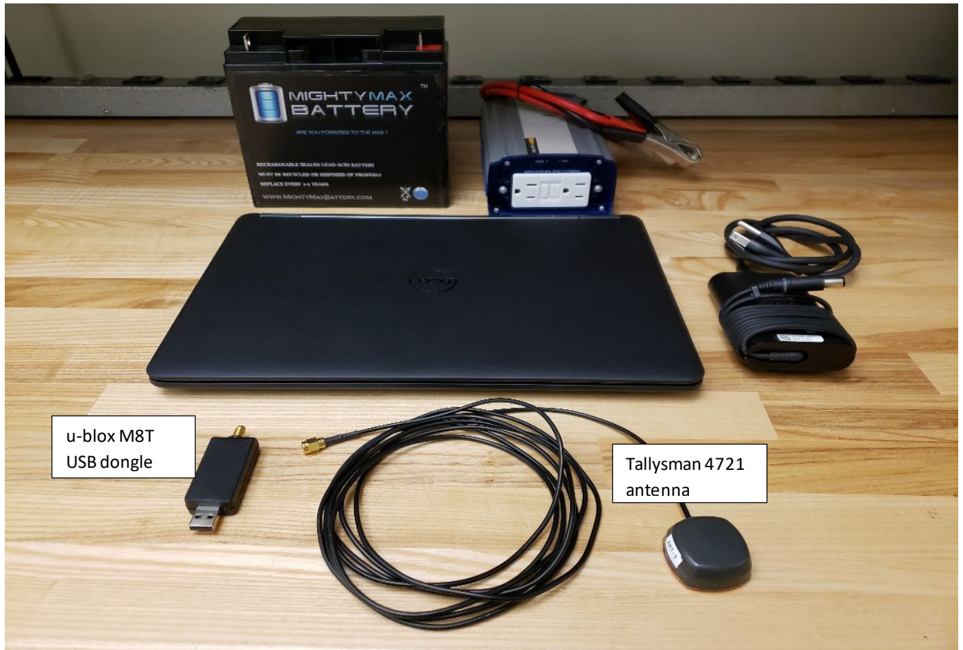
Figure 48 - START Base Station configuration featuring M8T dongle receiver and Tallysman 4721 active antenna
