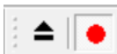
Figure 50 - Magnified view of Stop/Eject and Record buttons in u-center. The black Stop/Eject color indicates that data recording is active
