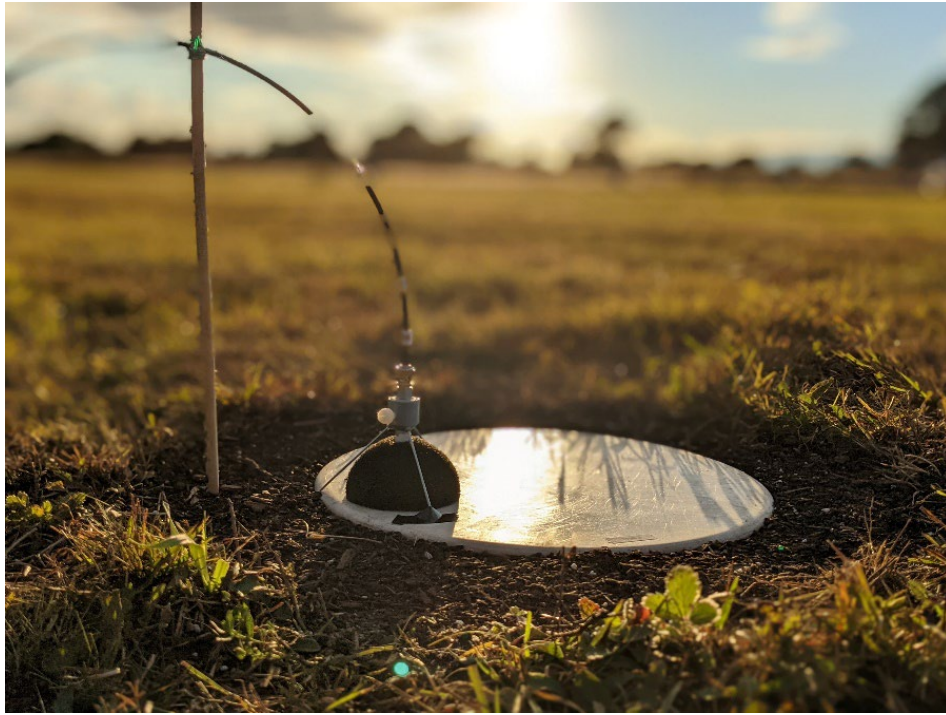
Figure 6 - Ground plate installation with microphone
