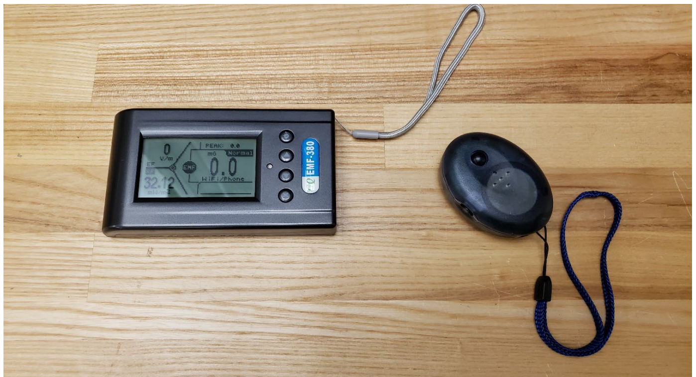
Figure 59 - EMI Detectors are helpful for identifying electro-magnetic "hotspots" during START Rover installations
