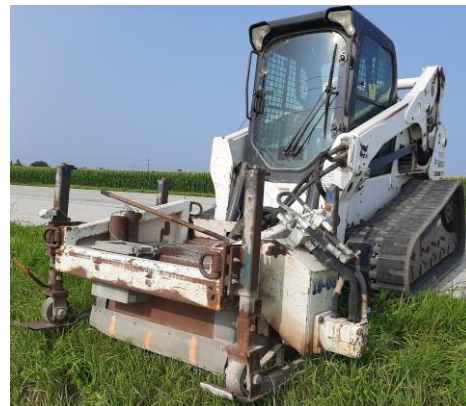
(b) Bobcat loader with asphalt planer
