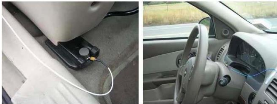
Figure 115. Photo. Accelerometer placement.
