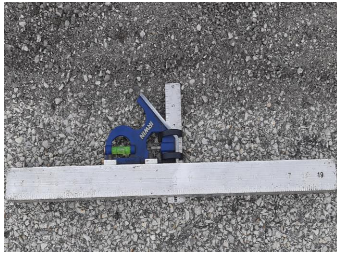
Figure 17. Photo. Ruler with depth gauge.
