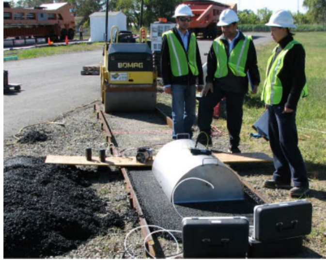
Figure E.7 Measuring VOCs using the transportable flux chamber (17)
