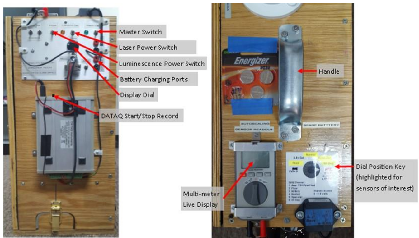
Figure 4-1: Diagram of box switchboard (left) and controls (right).
