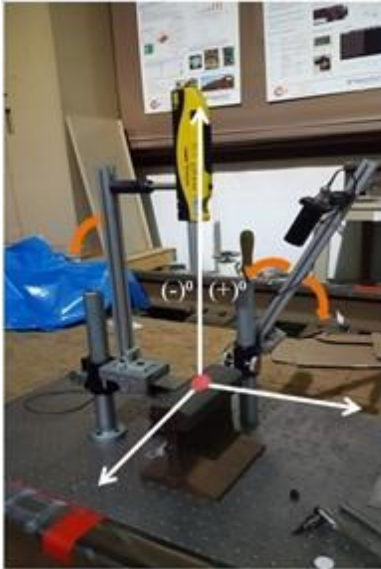
Figure 3-16: Separate laser emitter and receiver for out-of-plane experimental setup.
