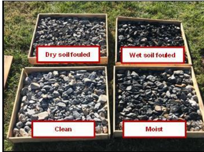
Figure 12 Ballast samples used in test A
