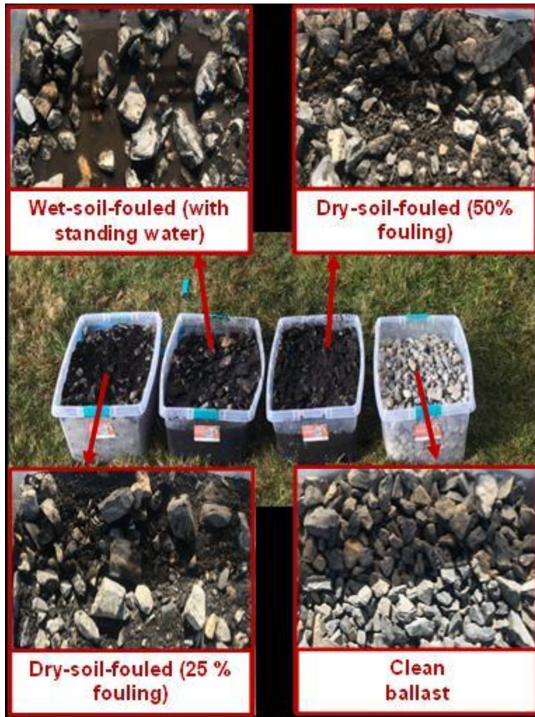
Figure 13. Ballast samples used in test B
