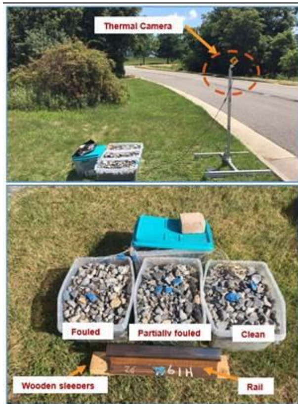
Figure 53 Measuring the temperature of the top surface of ballast by a thermal camera
