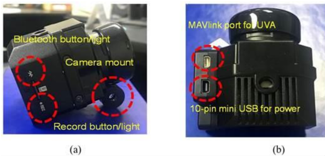
Figure 4 FLIR VUE PRO R (a) side view; (b) top view
