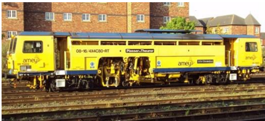
Figure 4 Tamping machine in operation (Plasser and Theurer 2010)
