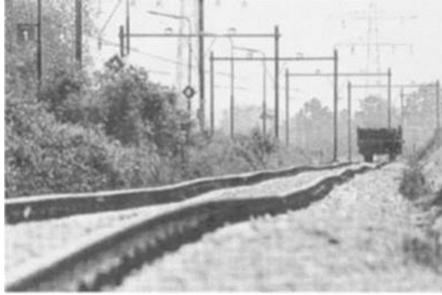
Figure 2 Defects in railway track geometry (Suiker 2002)
