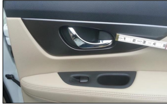
Figure 7. Second-row right door release lever and the rotating locking lever of an exemplar 2015 Nissan Rogue.
