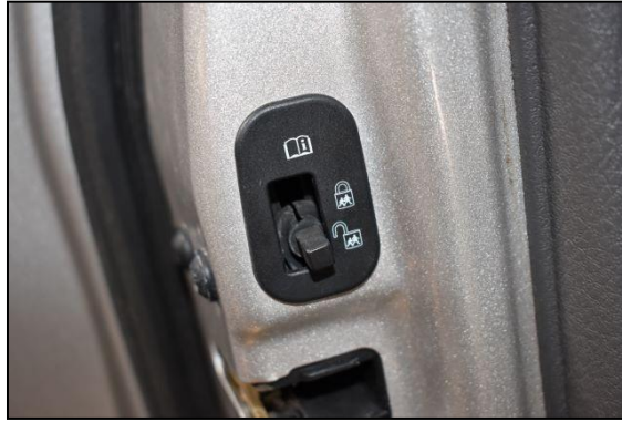
Figure 3. Child proof door lock, second-row left, 2002 Ford Explorer. Image obtained from local law enforcement.
