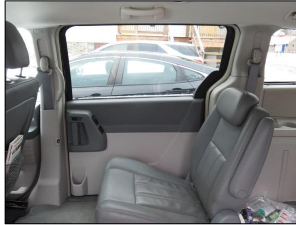
Figure 5. Second-row right interior door panel, door release lever and the lock lever of an exemplar vehicle
