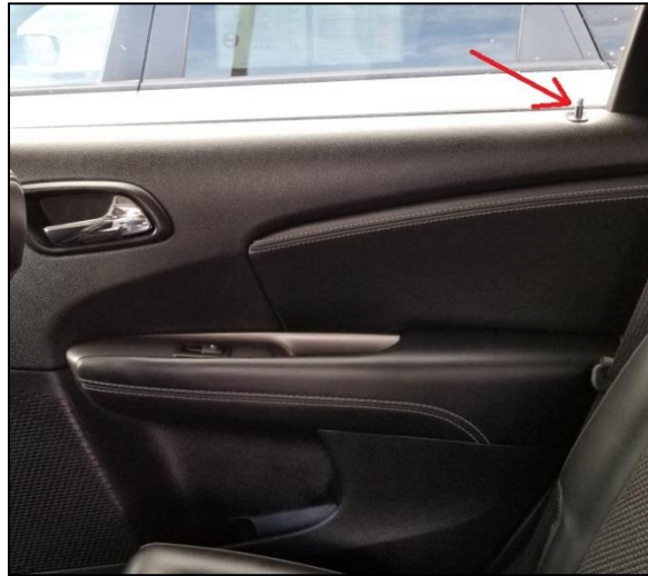
Figure 7. Lock stalk in unlocked position on the second-row right door of an exemplar Dodge
