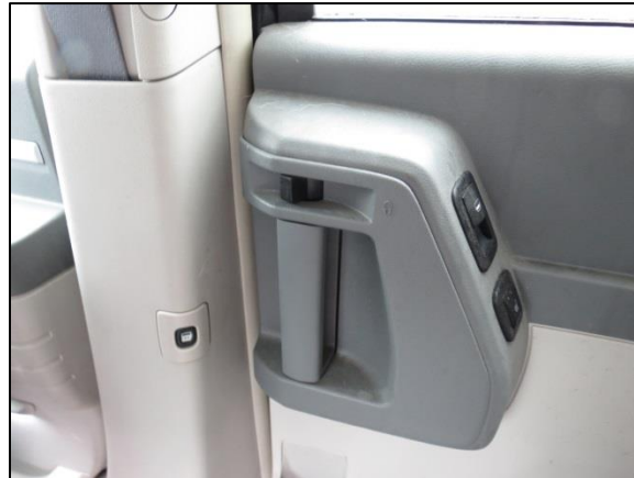
Figure 6. Door release lever and lock lever on right rear sliding door of an exemplar Dodge
