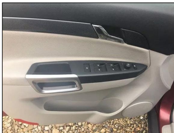
Figure 8. Power window and door lock switch console on the driver's door panel of an exemplar 2009 Saturn Vue XE
