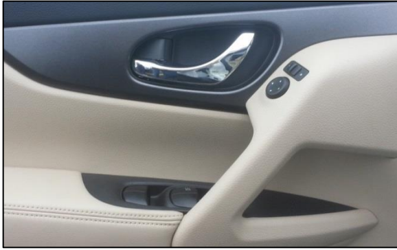
Figure 6. Front-row (driver's) door release lever and rotating locking lever in an exemplar 2015 Nissan Rogue.
