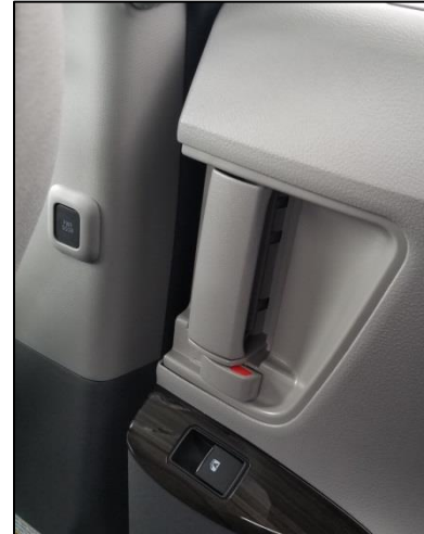
Figure 8. Close-up view of the interior locking system in the second row of an exemplar Toyota Sienna
