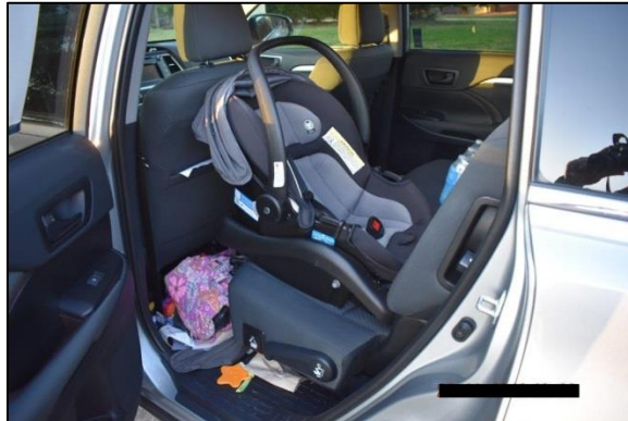
Figure 3. Installed position of the Safety First rear-facing CRS in the Toyota. Image provided by the investigating police department.
