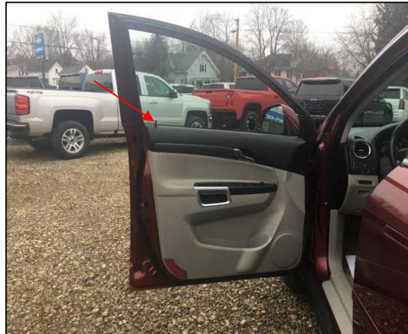
Figure 7. Driver's interior door release of an exemplar 2009 Saturn Vue XE
