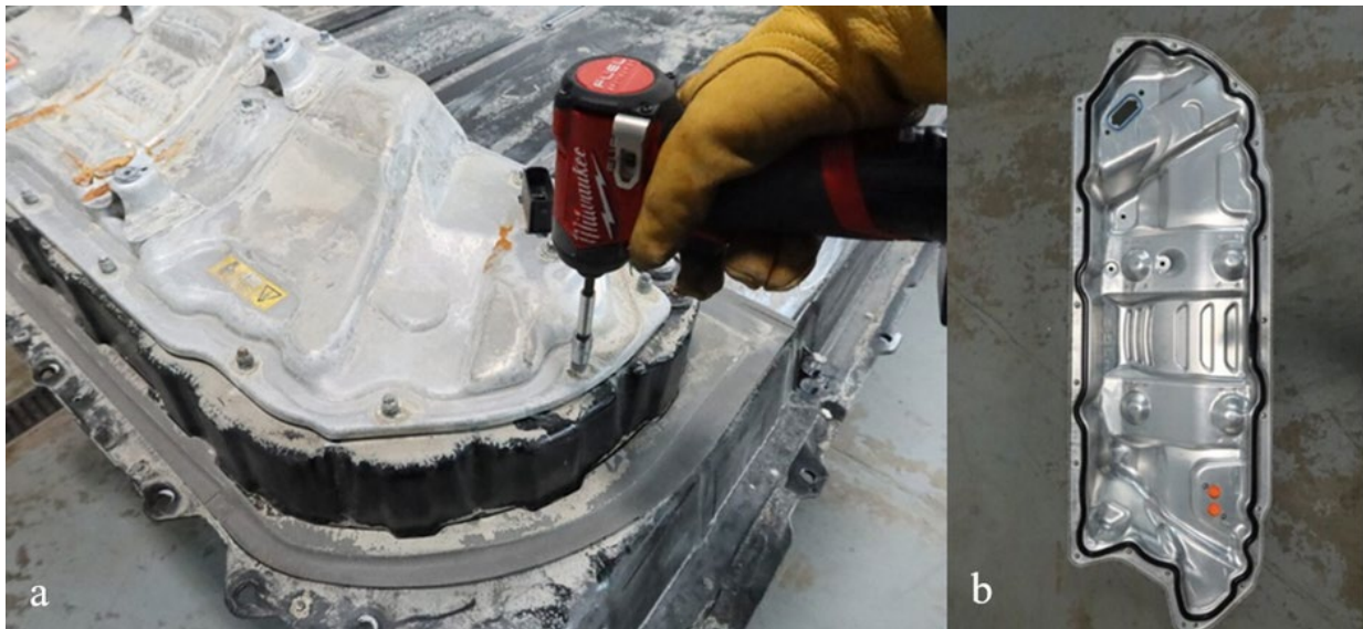
Figure 7. Pack Design 1 penthouse: (a) penthouse lid and (b) underside of penthouse lid, showing the reusable gasket
