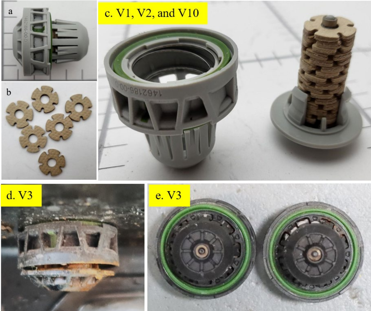
Figure 27. Penthouse moisture vents of Pack Design 1
