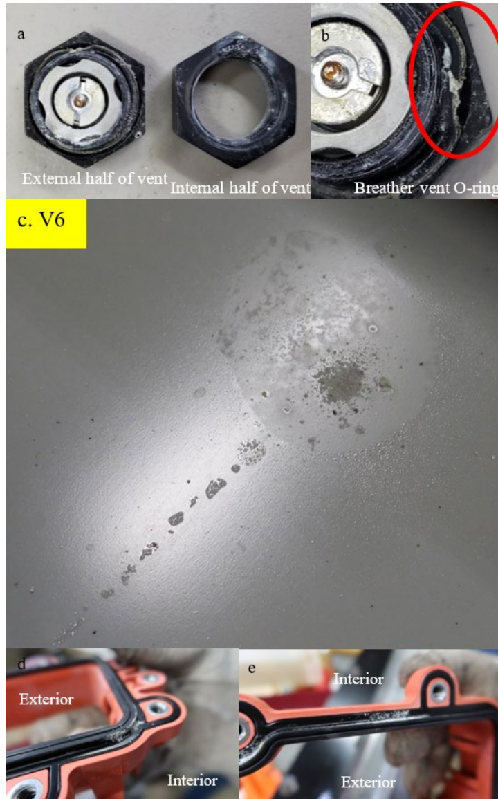
Figure 40. Vehicle V6 penthouse components: (a) exterior and interior of the penthouse breather vent, (b) compromised breather vent O-ring, (c) water marks and contaminants on the battery penthouse floor, directly underneath the breather vent, and (d, e) sediments on the pyrotechnic fuse
