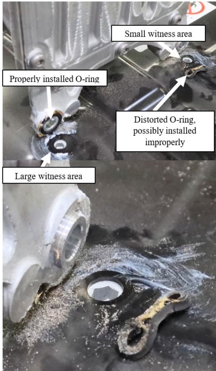
Figure 60. Possible assembly flaw found on the fastener seal of the electronics penthouse
