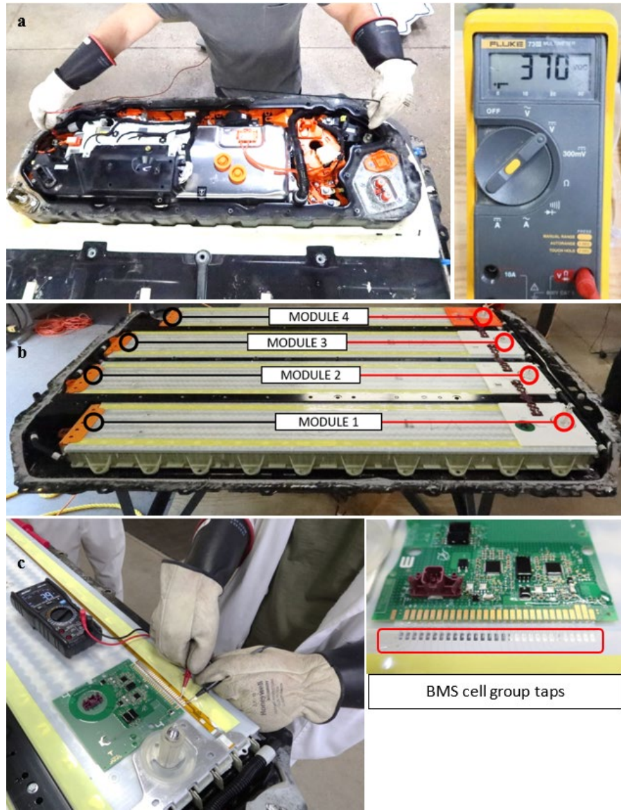
Figure 34. Inside of battery pack and measurement strategy: (a) pack voltage measurement through penthouse terminals, (b) module arrangement within a pack, and (c) cell group voltage measurement through BMS taps
