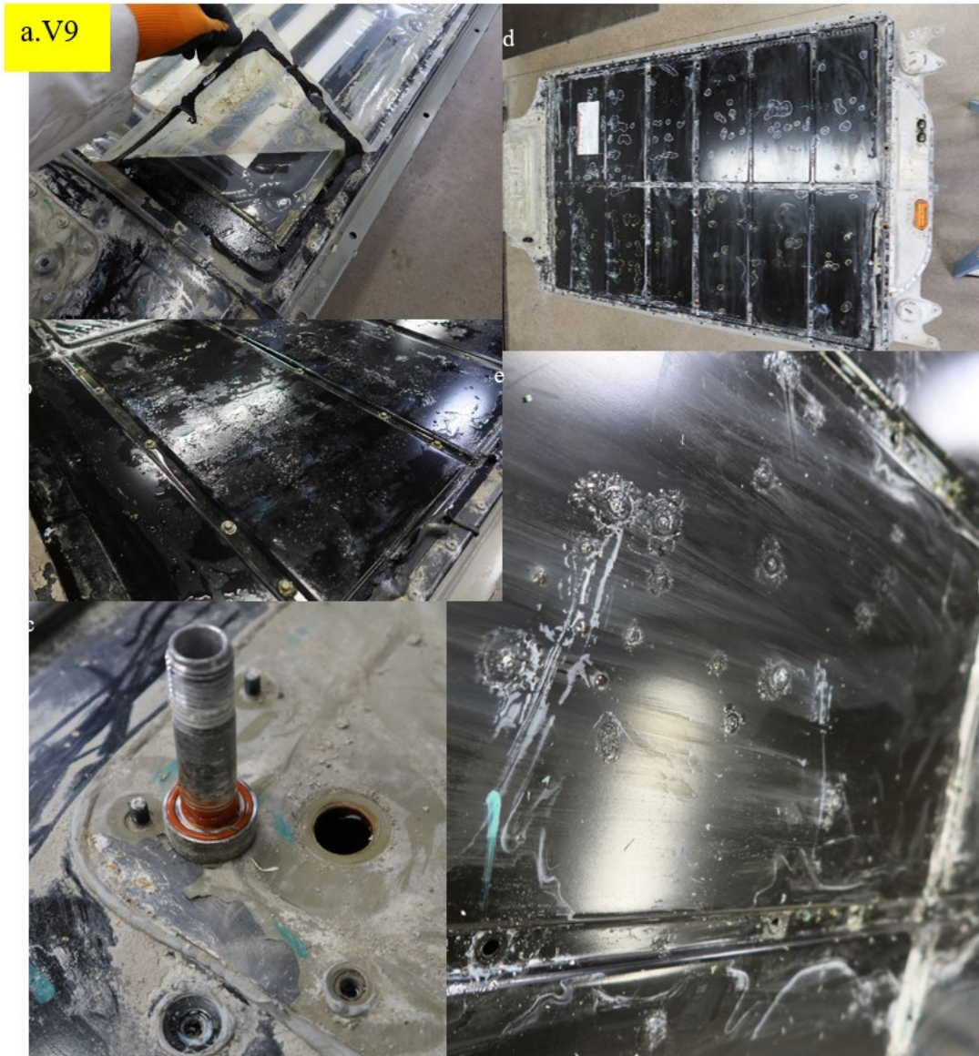
Figure 38. V9 battery pack after removal from the vehicle:
