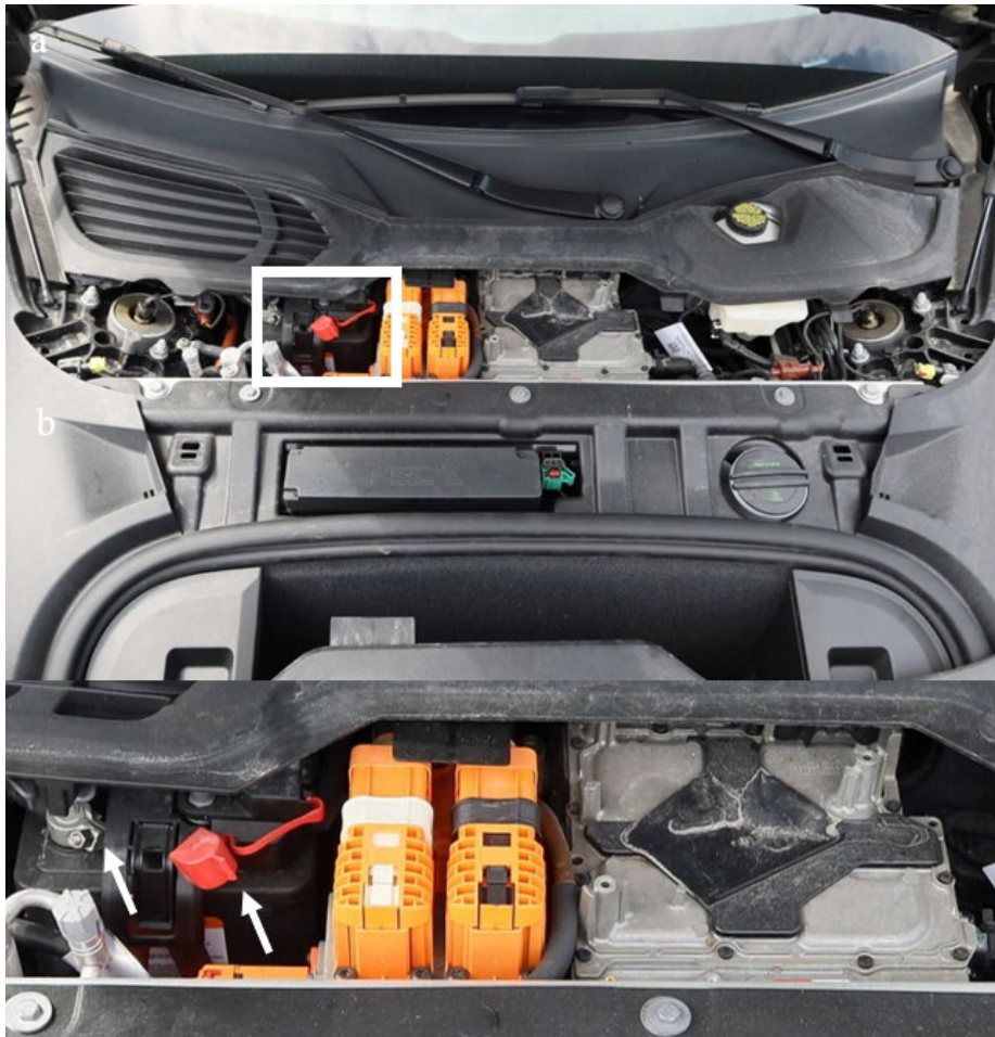
Figure 59. (a) 12-volt battery location and (b) 12-volt battery terminals, showing no corrosion
