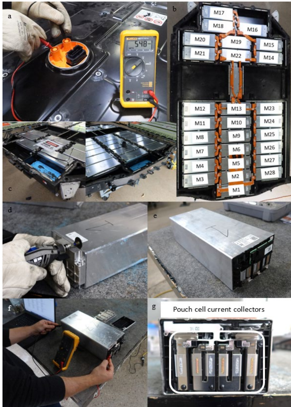
Figure 62. Porsche Taycan battery pack external and internal views with measurements being completed
