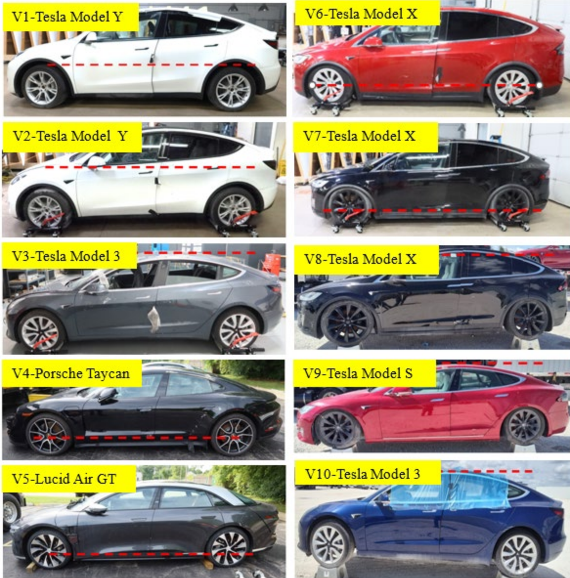
Figure 1. Ten flood-damaged EVs, showing the approximate flood-line represented by the dashed line
