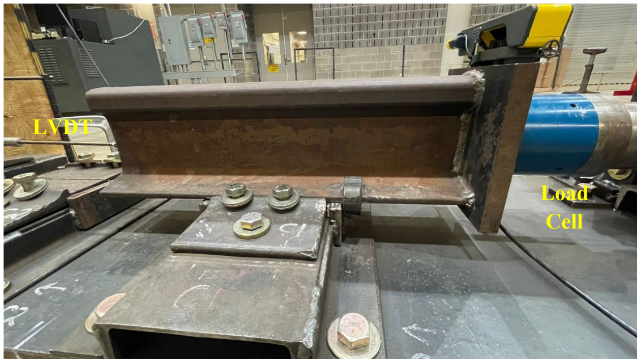
Figure 4: Side view of the rail with LVDT (left) and Load Cell (right)
