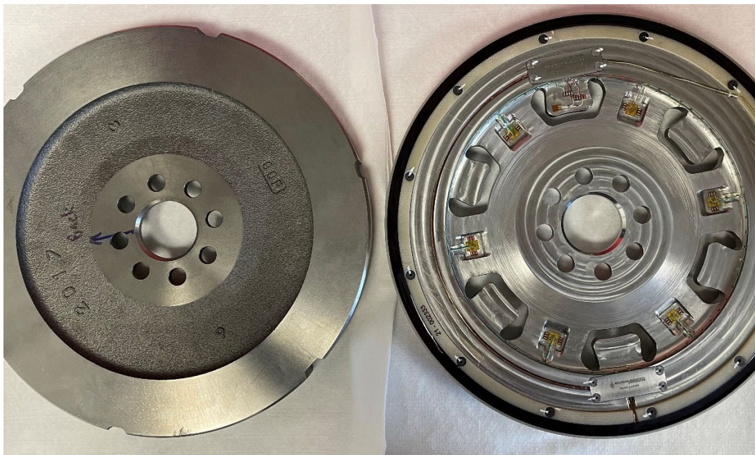
Figure 2. Stock flywheel and instrumented flywheel
