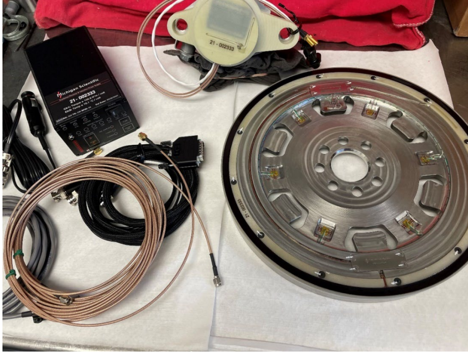
Figure 3. Michigan Scientific instrumented flywheel with instrumentation
