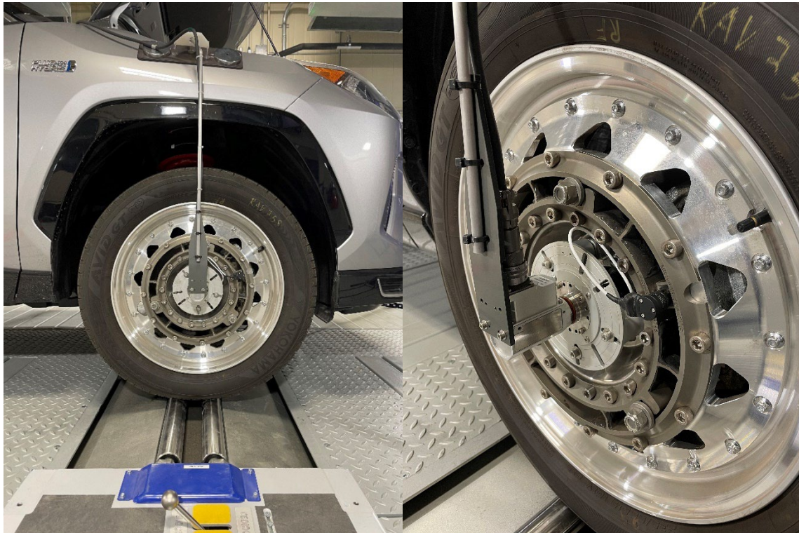
Figure 6. Torque wheel transducer installed on the Toyota RAV4
